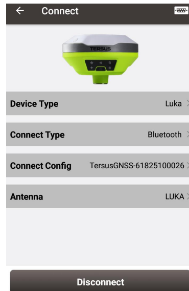
Figure 2.5 Connect LUKA via Bluetooth
