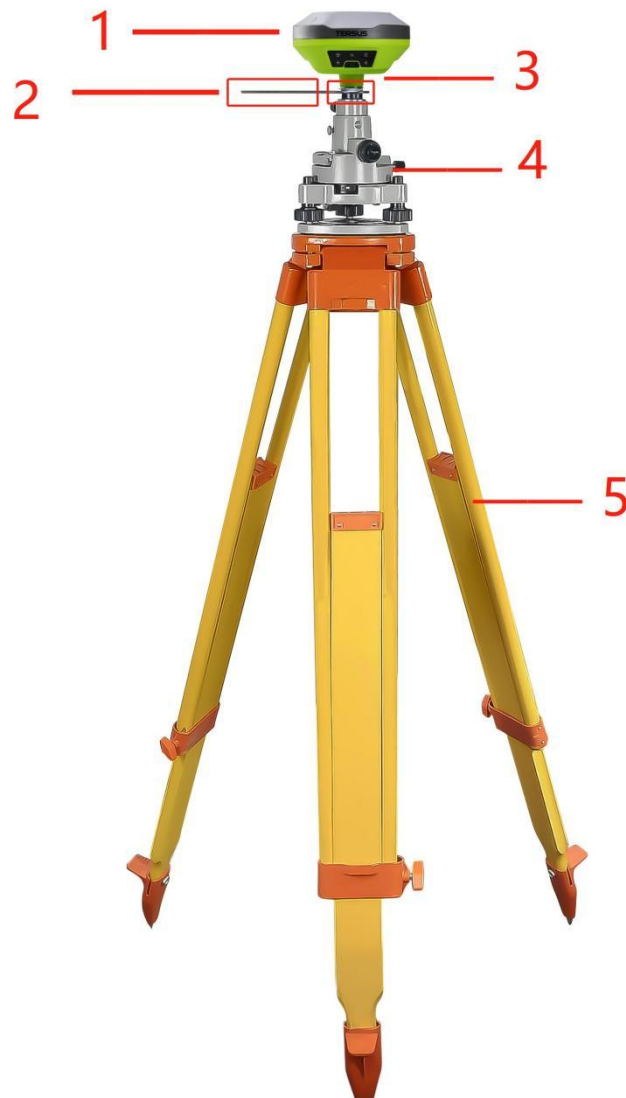
Figure 4.1 LUKA as a base - network mode
