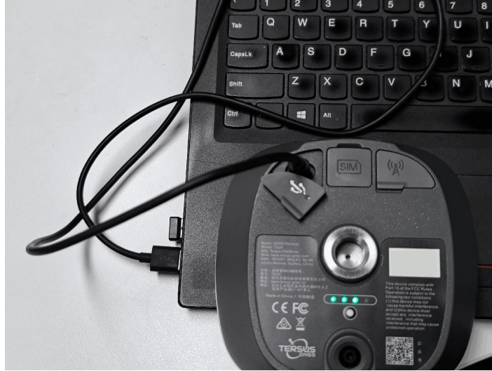
Figure 2.14 connect the computer and TS21
