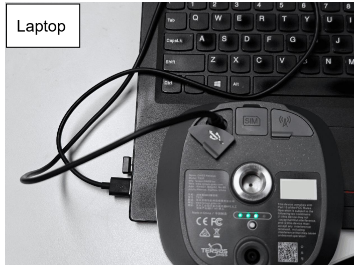
Figure 2.7 Connect TS21 to a computer
