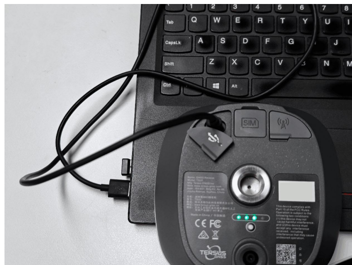
Figure 2.20 connect the computer and TS20
