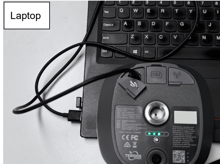
Figure 2.7 Connect TS20 to a computer
