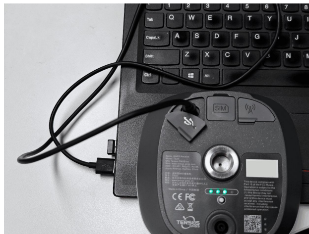
Figure 4 Type-C USB cable connect the computer and TS20 or TS21
