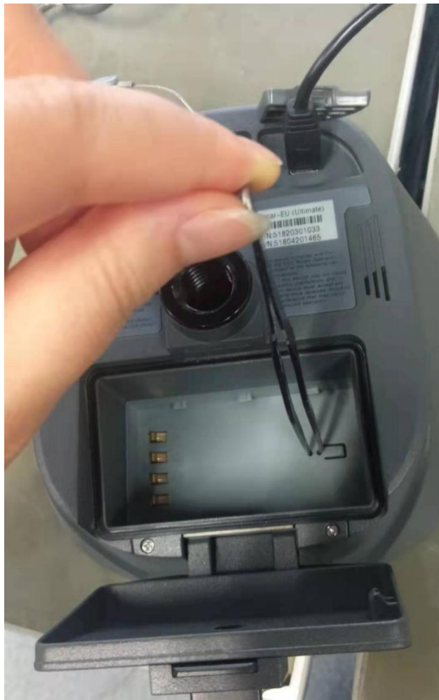
Figure7 the tweezers or metal cable touched the hole
