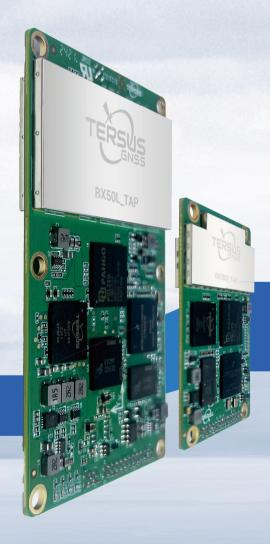
**GNSS OEM Boards & Module**
