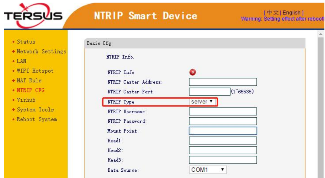
Figure 4.1 GeoBee30 under Ntrip server mode
