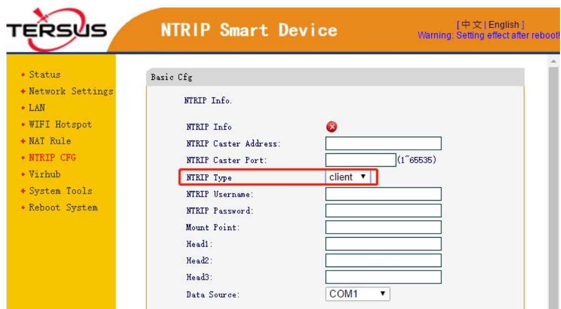
Figure 4.2 GeoBee30 under Ntrip client mode
