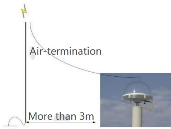
Figure 5.1 Schematic diagram of direct lightning prevention
