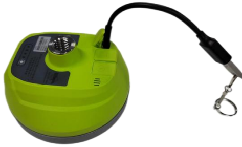
Figure 5 Connect LUKA to a USB flash drive
