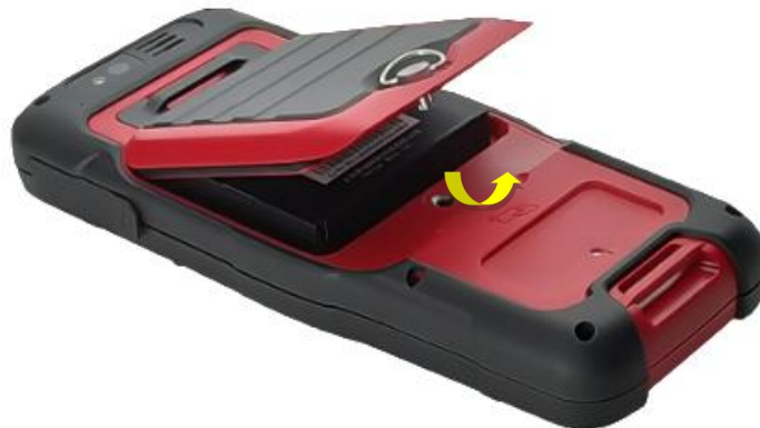
Figure 2.54 Take off the back cover
