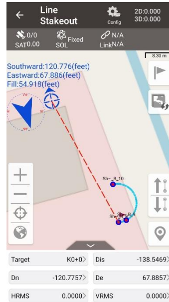
Figure 4.23 Stakeout an arc
