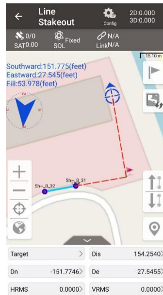
Figure 4.19 Stakeout a straight line
