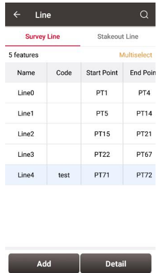
Figure 2.77 Survey line interface
