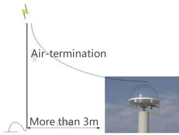
Figure 5.1 Schematic diagram of direct lightning prevention
