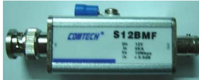
Figure 5.4 The lightning arrester for communication cable
