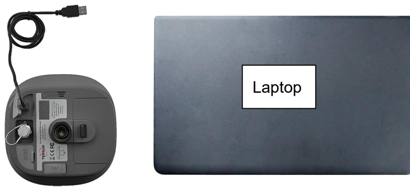
Figure 2.16 Connect Oscar to a computer
