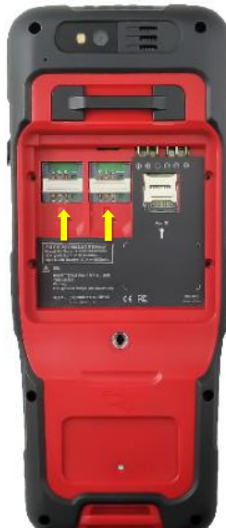
Figure 2.55 Put the SIM card in the holder
