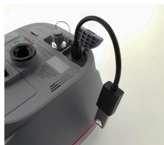
Figure 2.26 Connect Oscar to a USB flash drive
