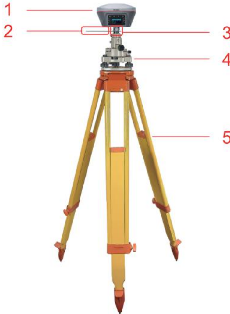
Figure 2.4 Oscar as a base without radio antenna
