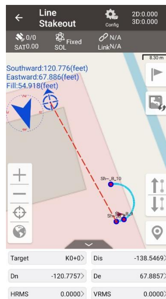
Figure 4.21 Stakeout an arc
