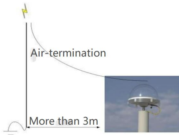
Figure 7.1 Schematic diagram of direct lightning prevention
