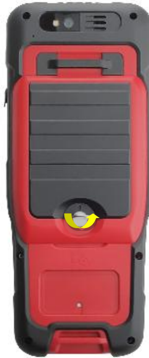
Figure 2.36 Remove the back cover
