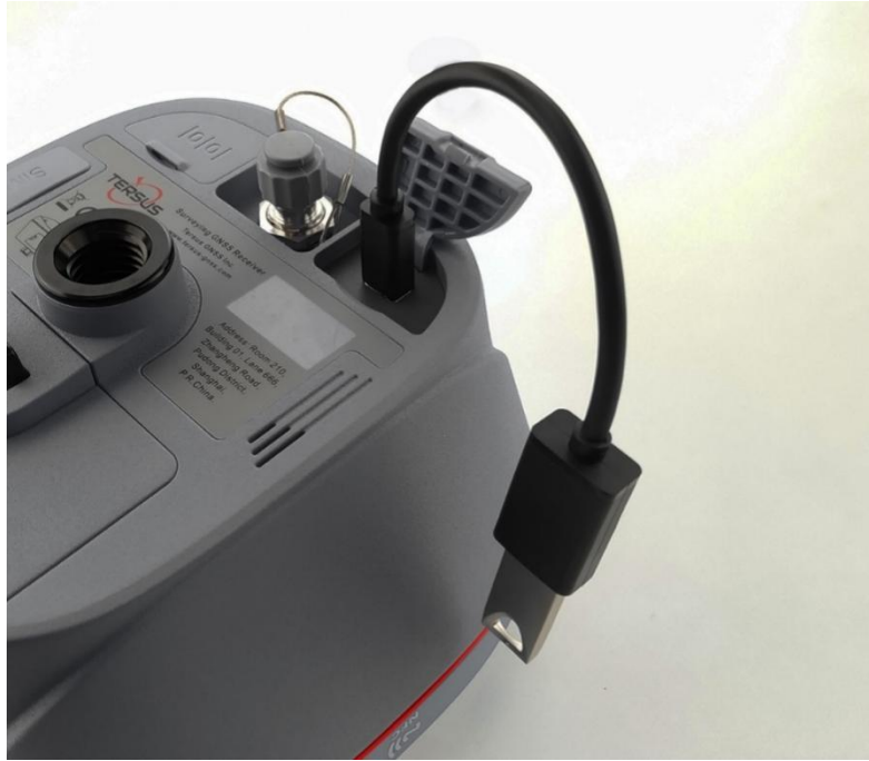
Figure 2.26 Connect Oscar to a USB flash drive
