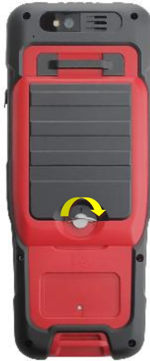
Figure 2.40 Insert the back cover
