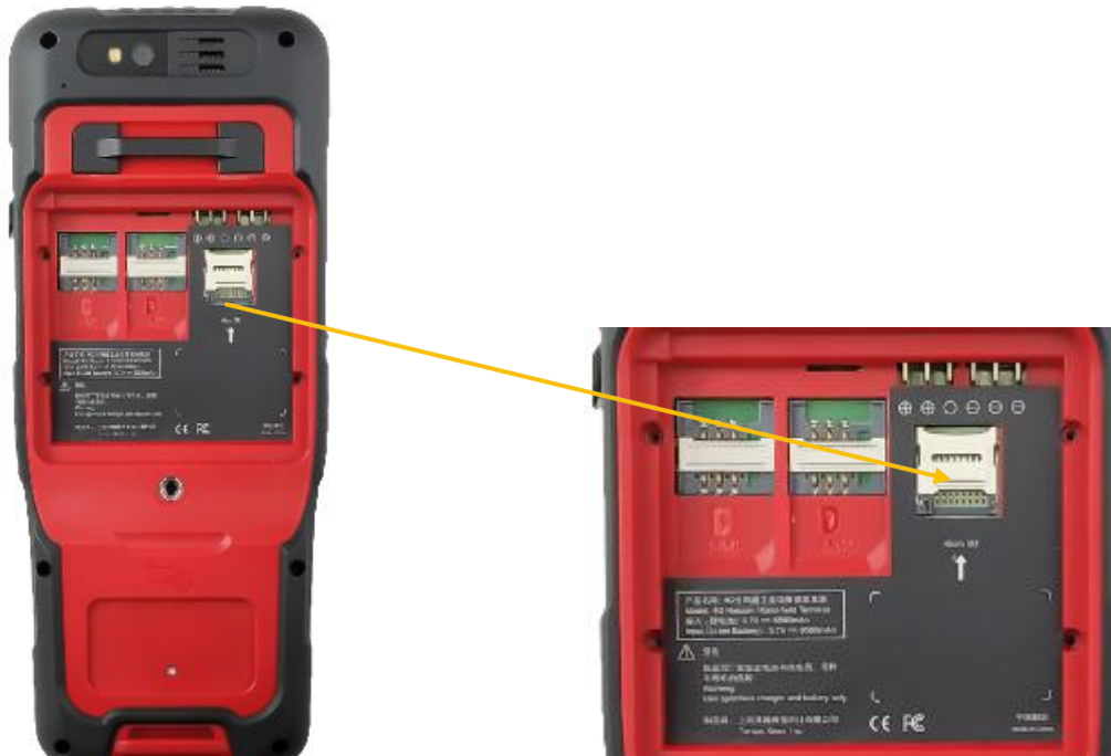
Figure 2.39 Insert Micro SD card
