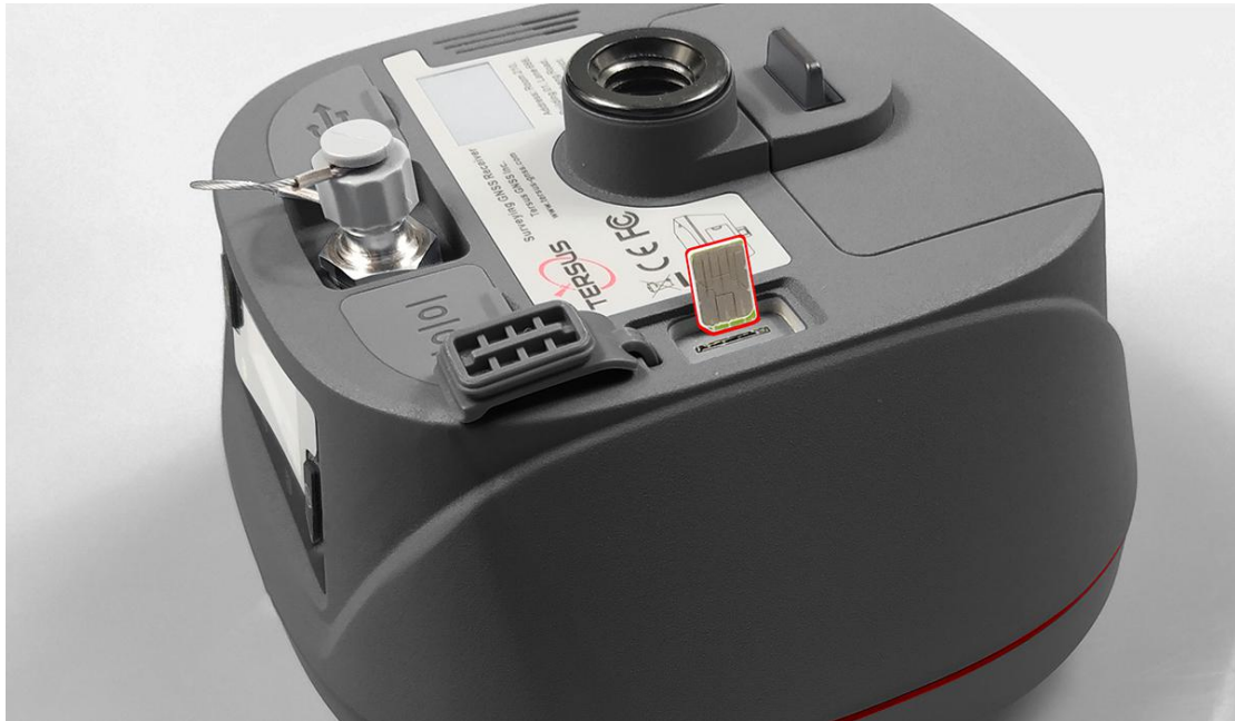
Figure 2.3 Insert the SIM card
