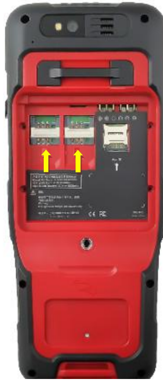
Figure 2.38 Put the SIM card in the holder
