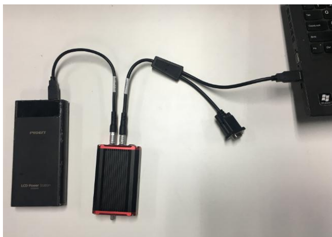
Figure 4.33 Connections of David, computer and power bank
