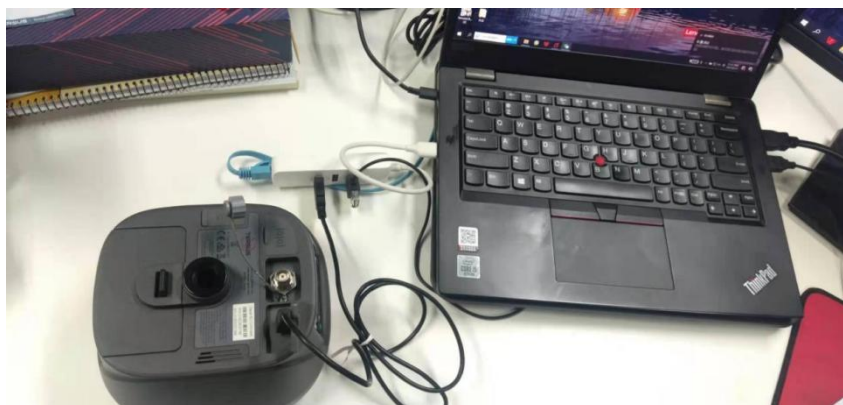
Figure 7 Mini USB cable connect the computer and OSCAR
