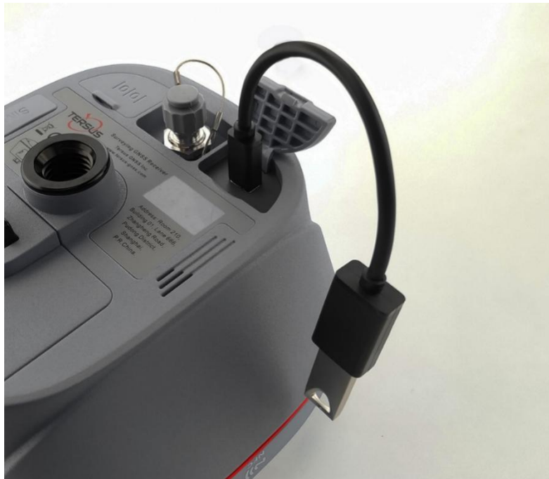
Figure 4 Connect Oscar to a USB flash drive
