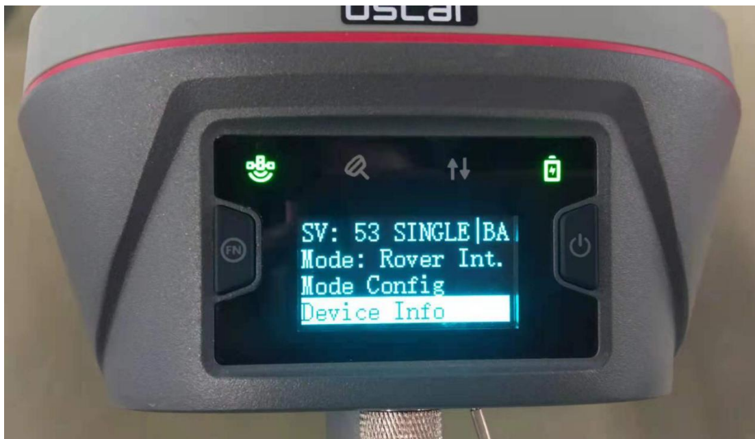
Figure 2.27 The LED panel displays the operation interface
