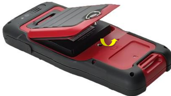
Figure 2.37 Take off the back cover
