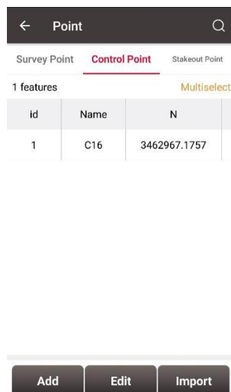
Figure 2.47 Control Point interface
