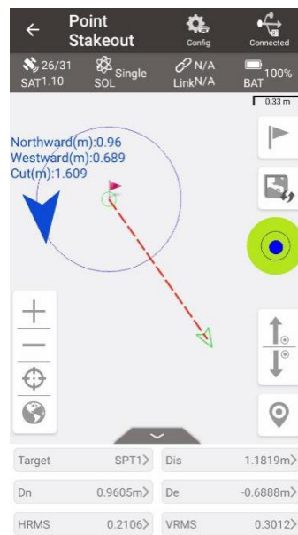
Figure 4.14 Point Stakeout interface
