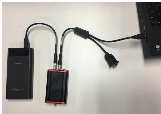
Figure 4.33 Connections of David, computer and power bank
