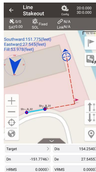
Figure 4.17 Stakeout a straight line
