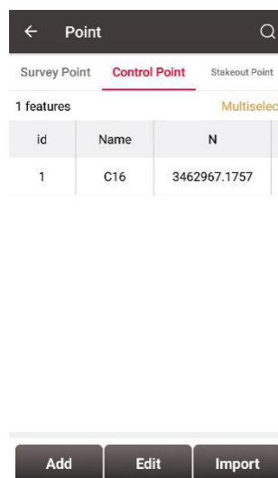
Figure 2.53 Control Point interface
