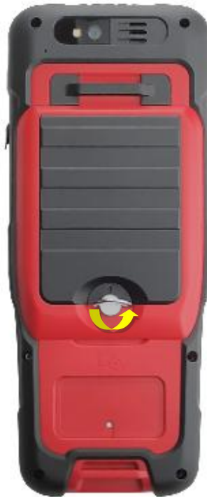
Figure 6.8 Remove the back cover
