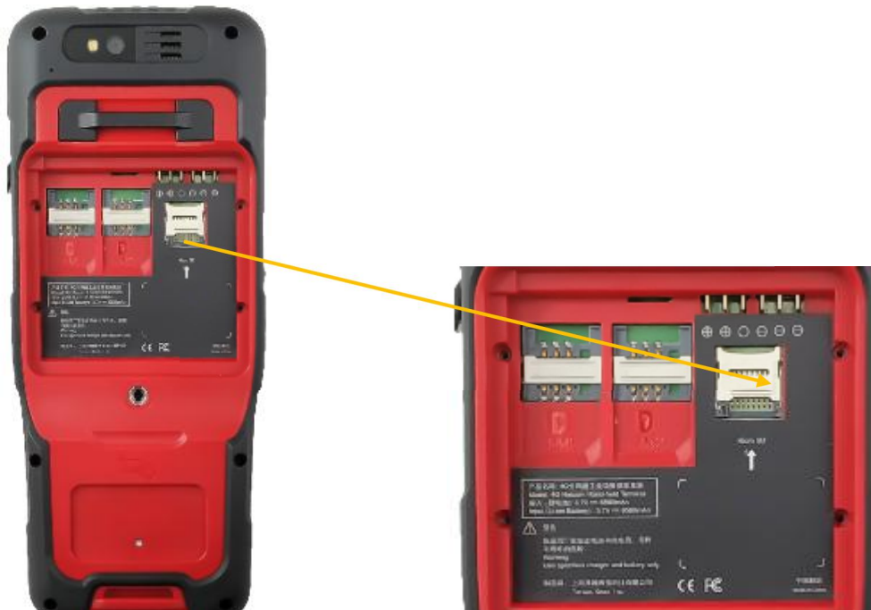
Figure 6.11 Insert Micro SD card
