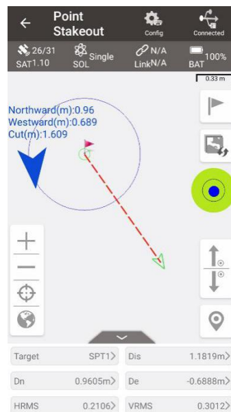
Figure 4.14 Point Stakeout interface
