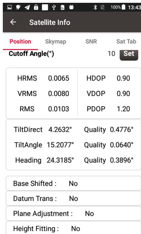
Figure 4.26 Detailed information of tilt compensation
