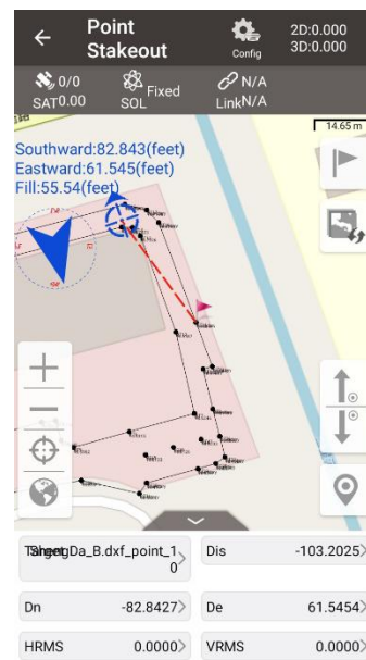
Figure 4.7 Switch to point stakeout
