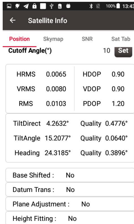
Figure 4.19 Detailed information of tilt compensation
