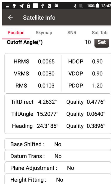
Figure 4.17 Detailed information of tilt compensation
