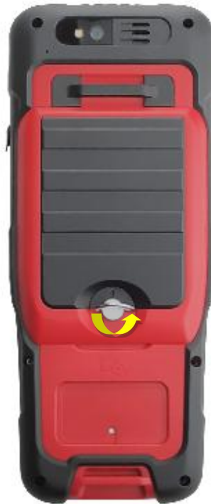
Figure 6.8 Remove the back cover
