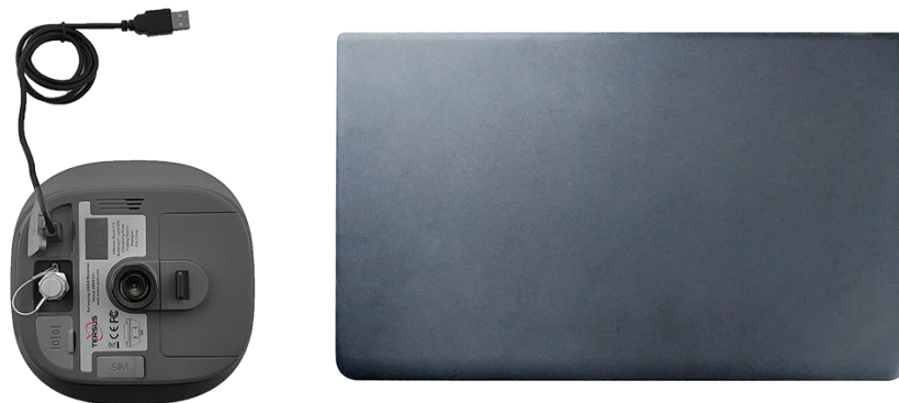
Figure 4.29 Connect Oscar to a computer
