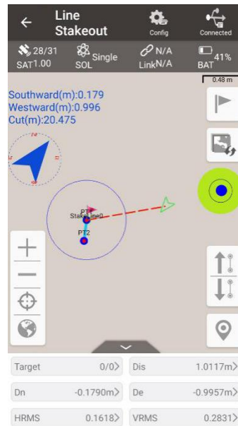
Figure 4.14 Line Stakeout interface
