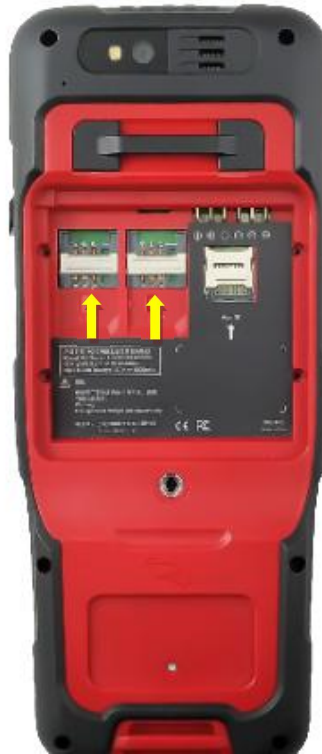
Figure 6.10 Put the SIM card in the holder
