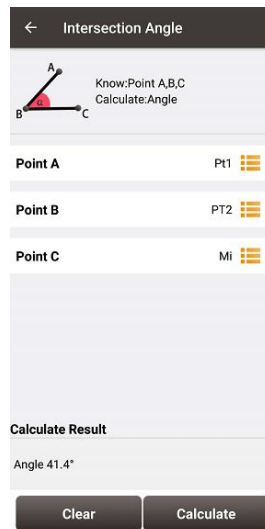
Figure 5.15 Intersection Angle calculation
