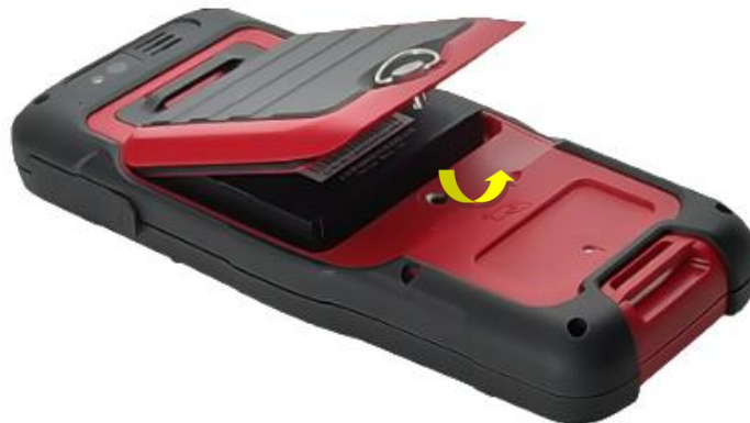
Figure 2.20 Take off the back cover
