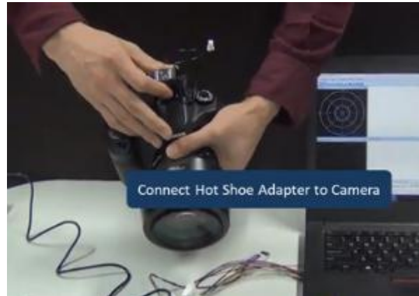
Figure 2.3 Connect hot shoe adapter to the camera
