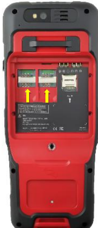
Figure 6.10 Put the SIM card in the holder
