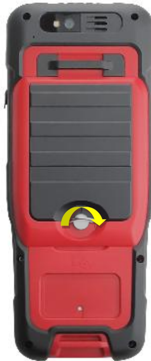
Figure 6.12 Insert the back cover
