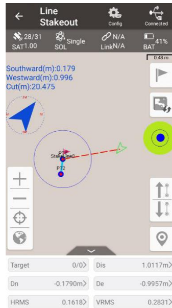
Figure 4.14 Line Stakeout interface
