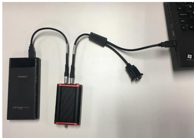
Figure 4.24 Connections of David, computer and power bank
