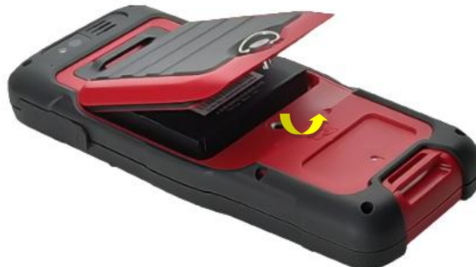
Figure 6.9 Take off the back cover
