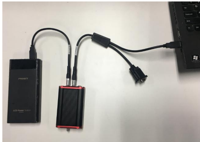
Figure 4.22 Connections of David, computer and power bank
