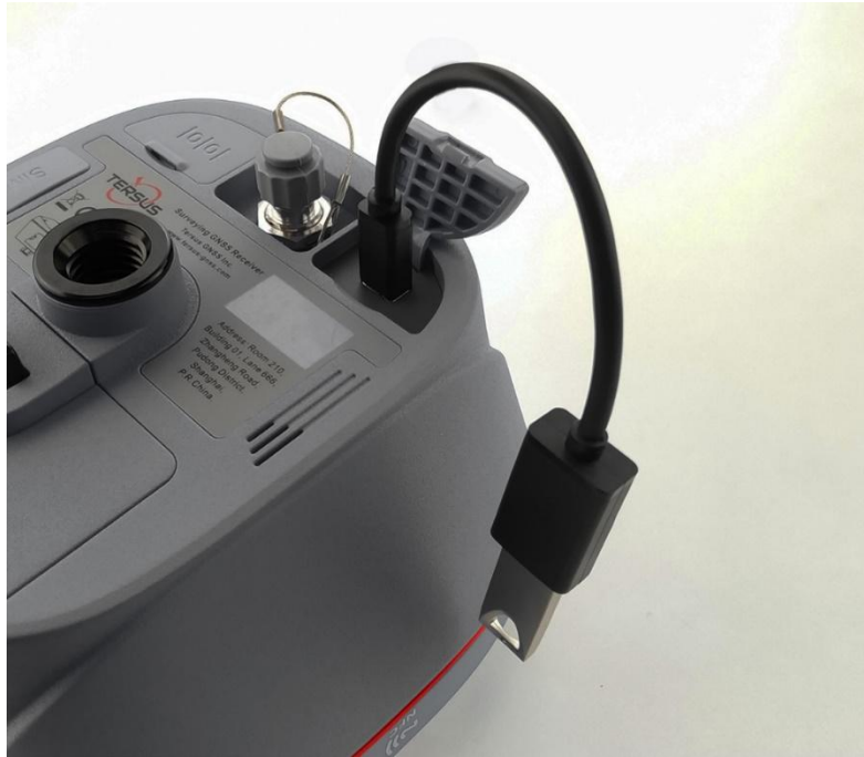
Figure 3 Connect Oscar to a USB flash drive
