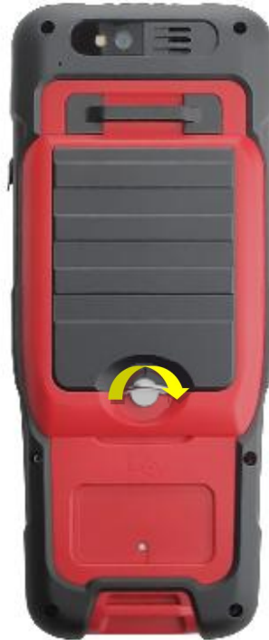
Figure 6.12 Insert the back cover
