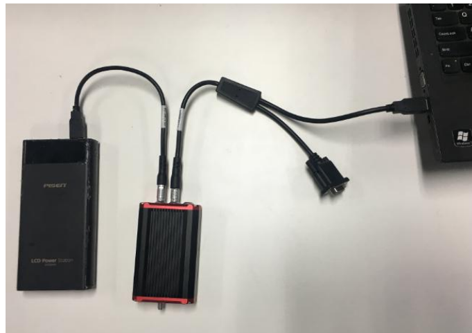
Figure 4.16 Connections of David, computer and power bank
