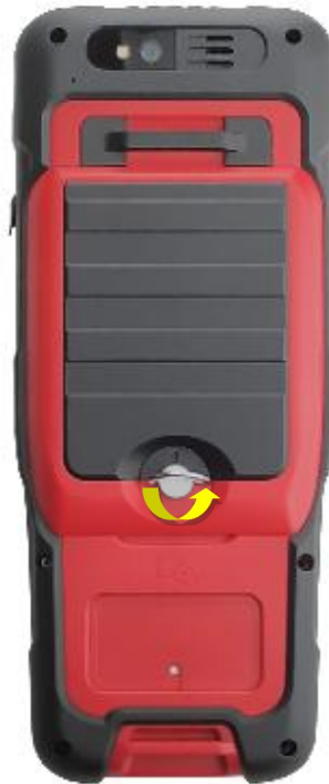
Figure 6.8 Remove the back cover
