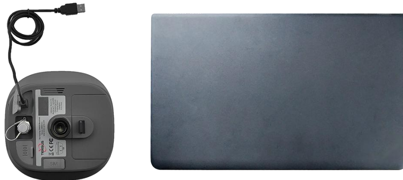
Figure 4.21 Connect Oscar to a computer
