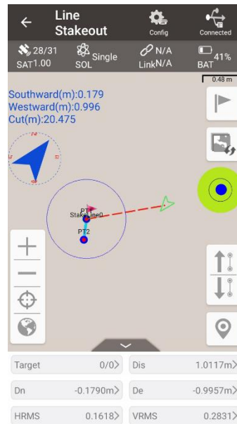
Figure 4.10 Line Stakeout interface
