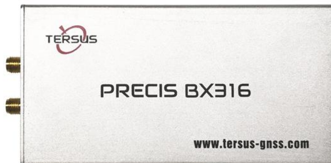
Figure 1.13 Overview of BX316 Enclosure
