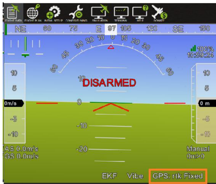
Figure 5.26 GPS status changes to rtk Fixed
