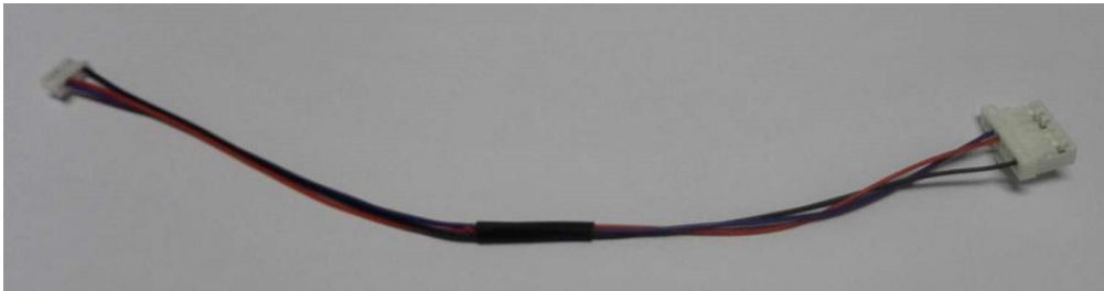
Figure 5.22 Cable between Pixhawk and BX306
