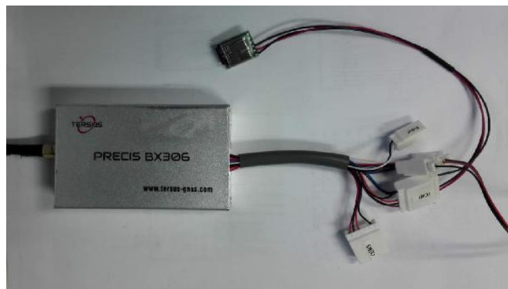
Figure 5.15 Outline of BX306 Connected to DL207
