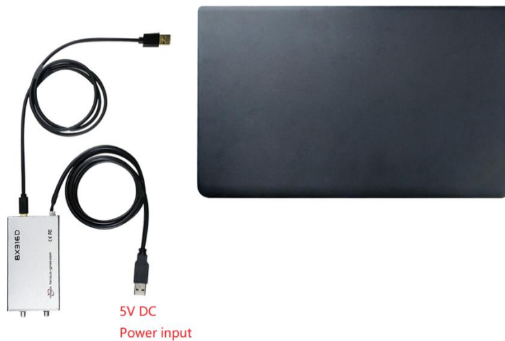
Figure 2.10 BX316D Enclosure connected to a Laptop
