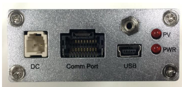
Figure 1.17 BX316D Enclosure Panel
