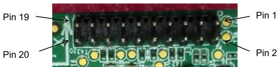
Figure 4.8 Connector J3 of BX316D
