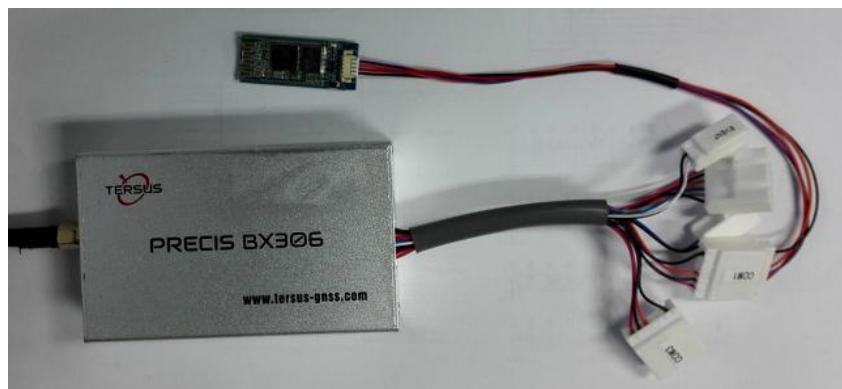
Figure 5.9 Outline of BX306 Connected to BT120
