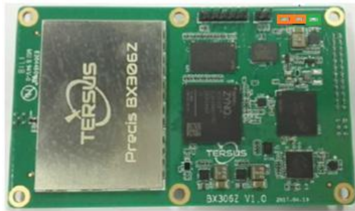
Figure 1.4 The other side of BX306Z Board
