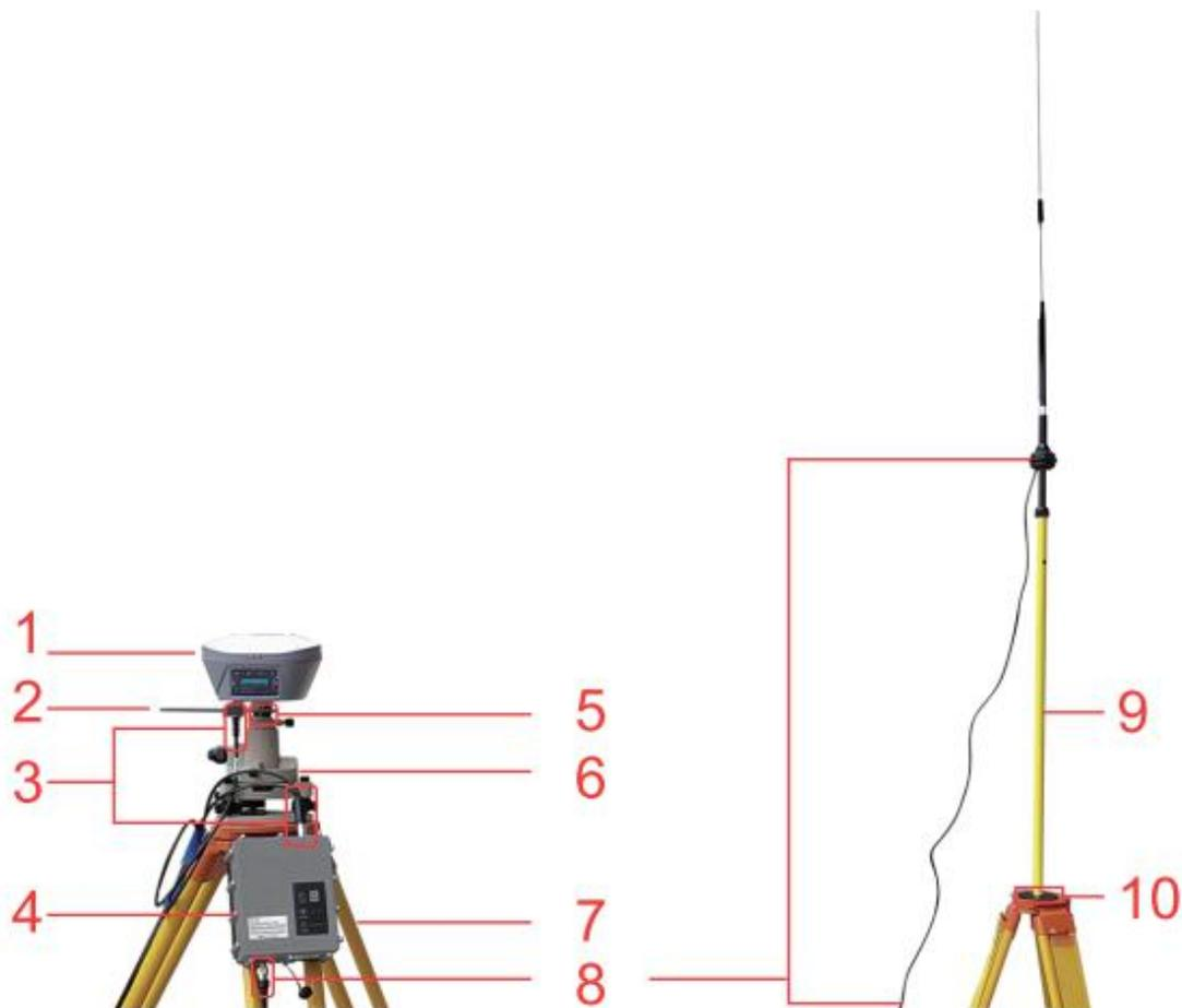
Figure 4.3 Oscar as a Base - External 25W Radio
