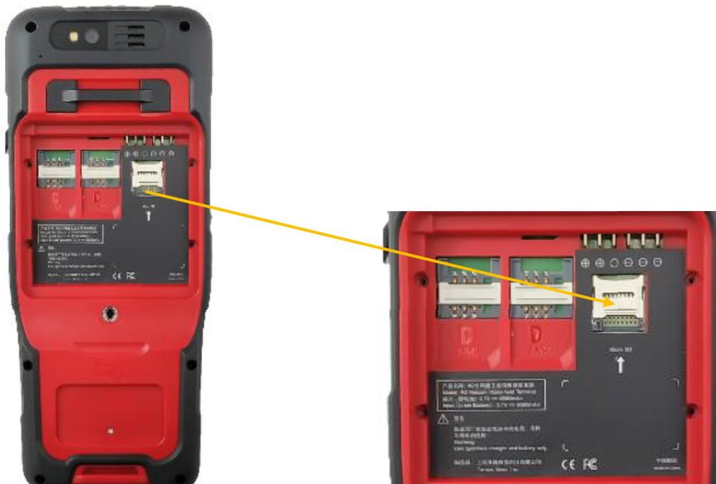
Figure 2.17 Insert T-Flash card
