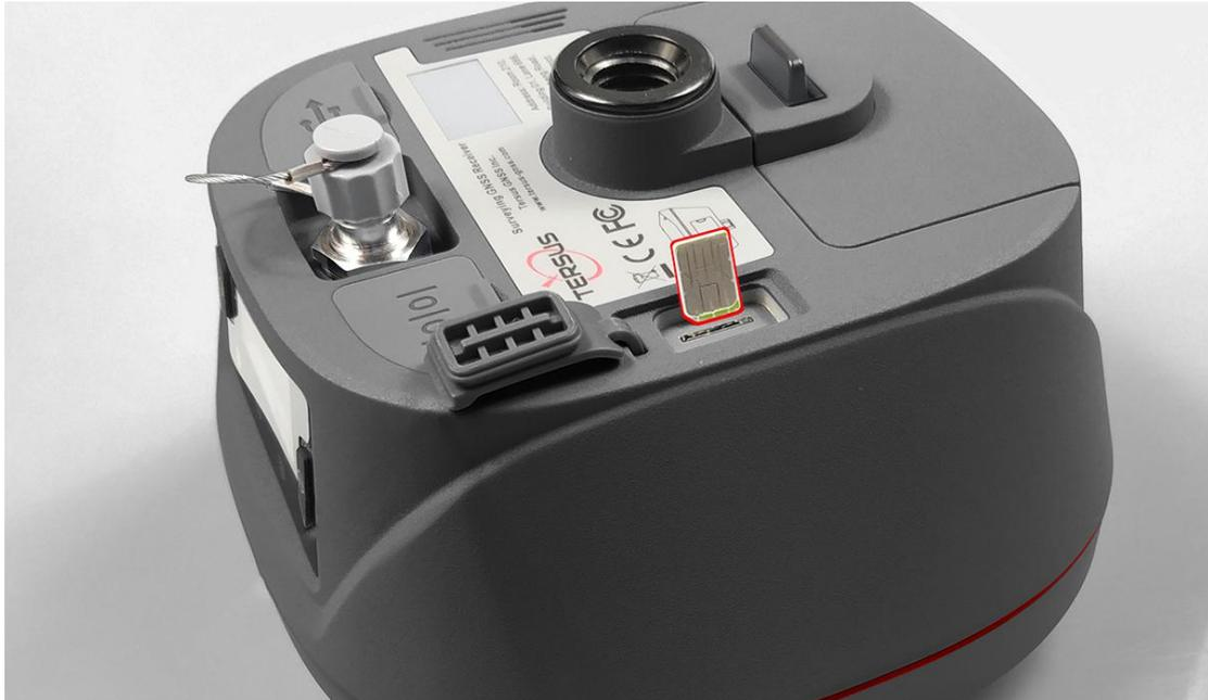
Figure 2.3 Insert the SIM card
