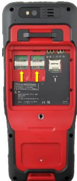
Figure 2.16 Put the SIM card in the holder
