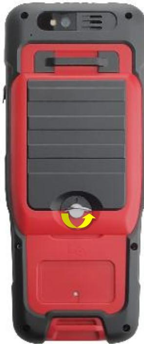
Figure 2.14 Remove the back cover
