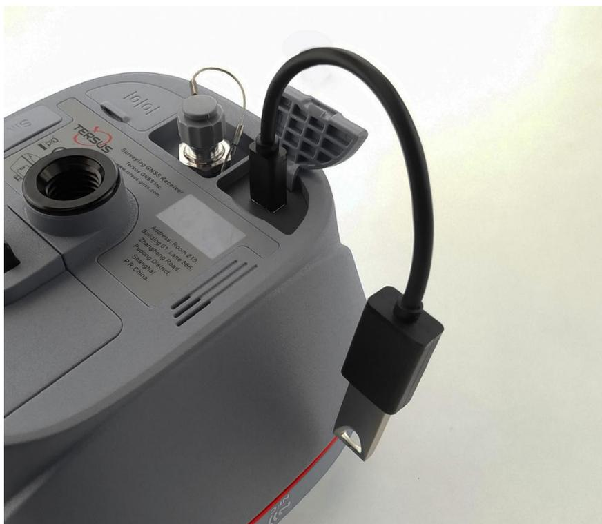
Figure 2.13 Connect Oscar to a USB memory stick
