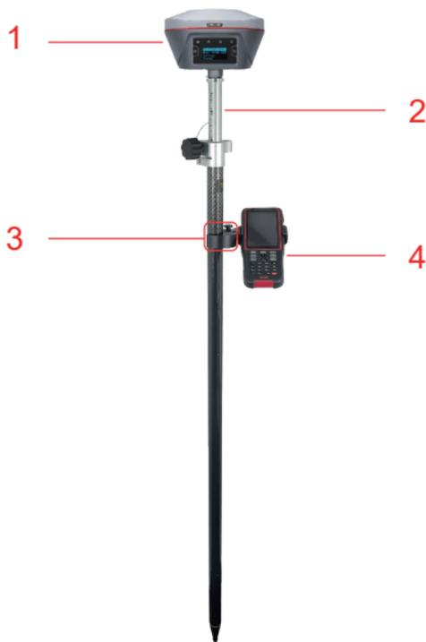
Figure 1.4 Oscar as a Rover – Network Mode
