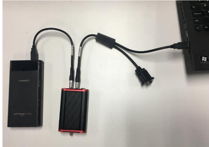
Figure 7.2 Connections of David, computer and power bank
