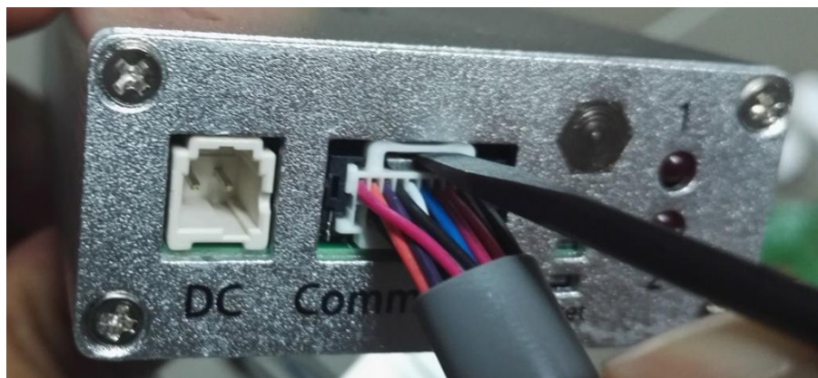
Figure 5.28 Uninstall the Cable
