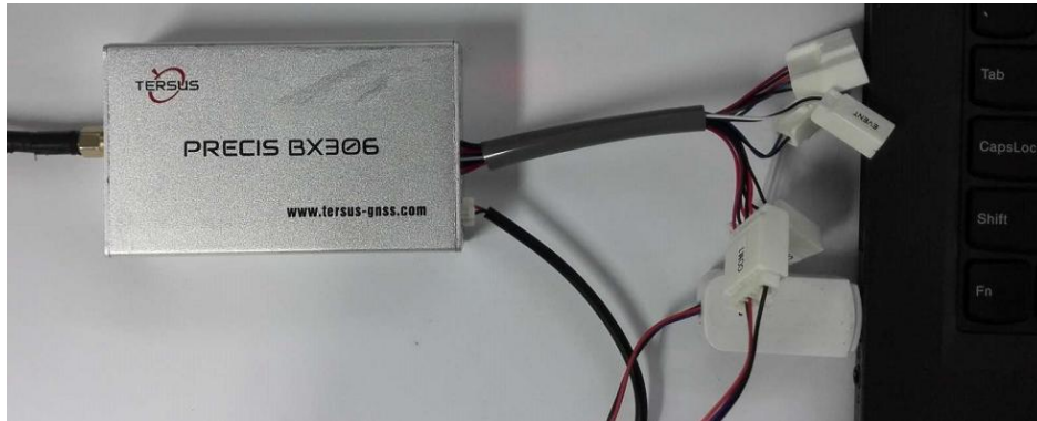
Figure 2.10 BX306 Enclosure Connected to a Laptop
