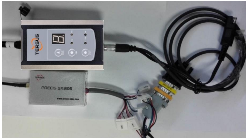
Figure 5.21 Outline of BX306 Connected to RS460 Radio
