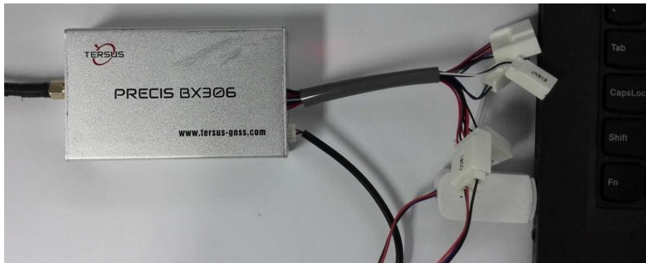
Figure 2.10 BX306 Enclosure Connected to a Laptop
