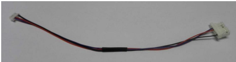
Figure 5.22 Cable between Pixhawk and BX306
