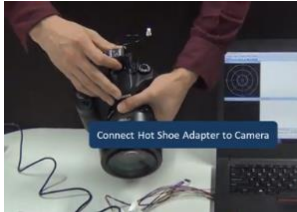
Figure 2.3 Connect hot shoe adapter to the camera
