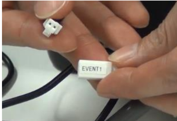
Figure 2.5 Connect hot shoe connector to the EVENT connector
