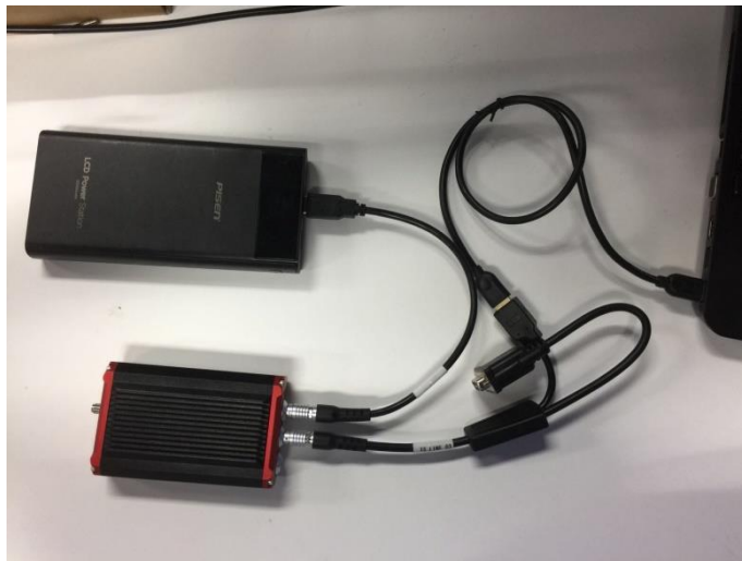
Figure 6.2 Connections of David, computer and power bank
