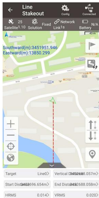
Figure 4.6 Line Stakeout interface
