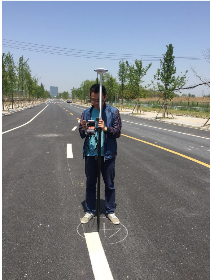
Figure 4 Surveying the GCPs
