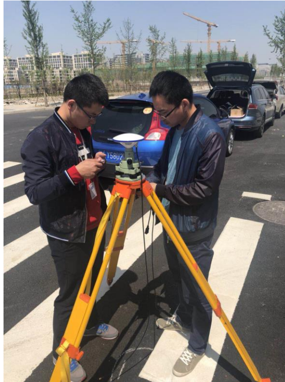
Figure 7 Base Station Recording GNSS Data
