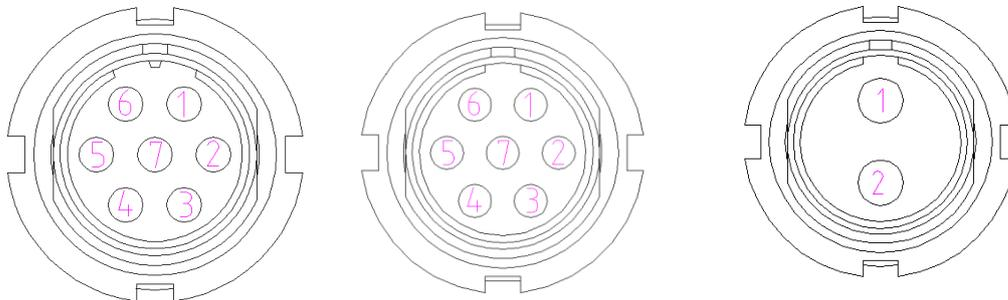
Figure 53 Pin Definition of the COMM1/COMM2/DC ports
