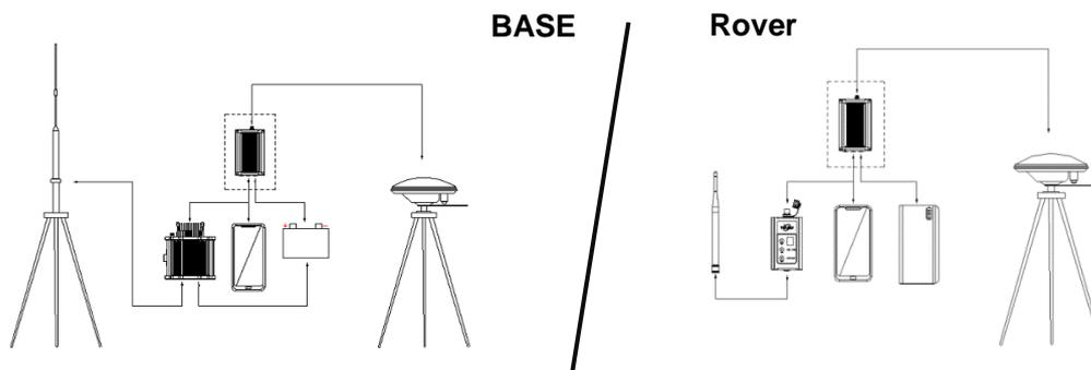
Figure 56 Outline of Base/Rover with Radios
