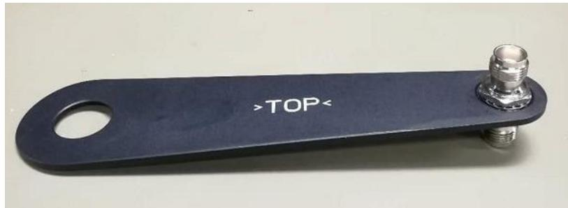
Figure 28 TNC - TNC converter & Bracket for 460M antenna
