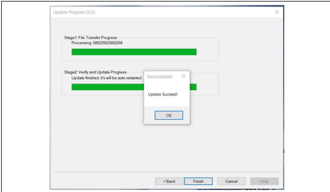
6. Press OK and Finish buttons to close the FW upgrade windows, the receiver will reset automatically.
