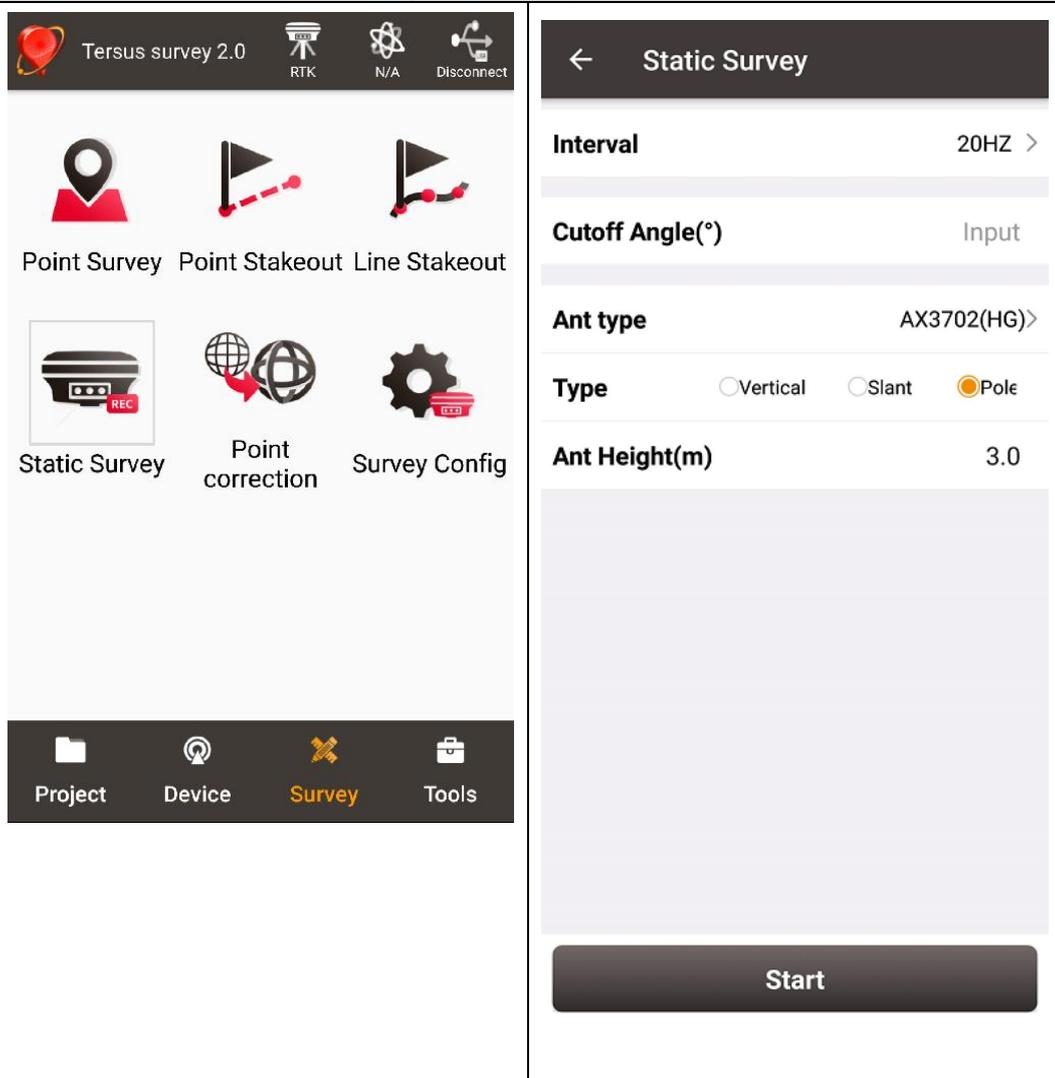
6. Ensure the necessary parameters, including data frequency and cutoff angle, etc. Press Start.
