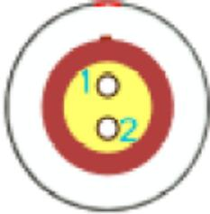
A diagram of a circular power input port. It features a central yellow circle with two small white circles inside, labeled '1' and '2' in blue. This is surrounded by a red ring, which is further enclosed by a white ring. The entire assembly is within a larger white circle. | Pin 1: GND<br>Pin2: PWR input |
