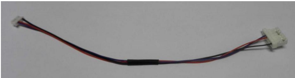
Figure 27 Cable between Pixhawk and BX306
