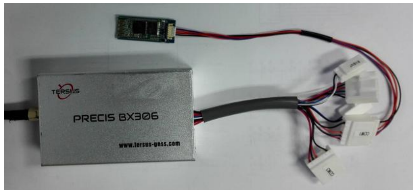
Figure 35 Outline of BX306 Connected to BT120
