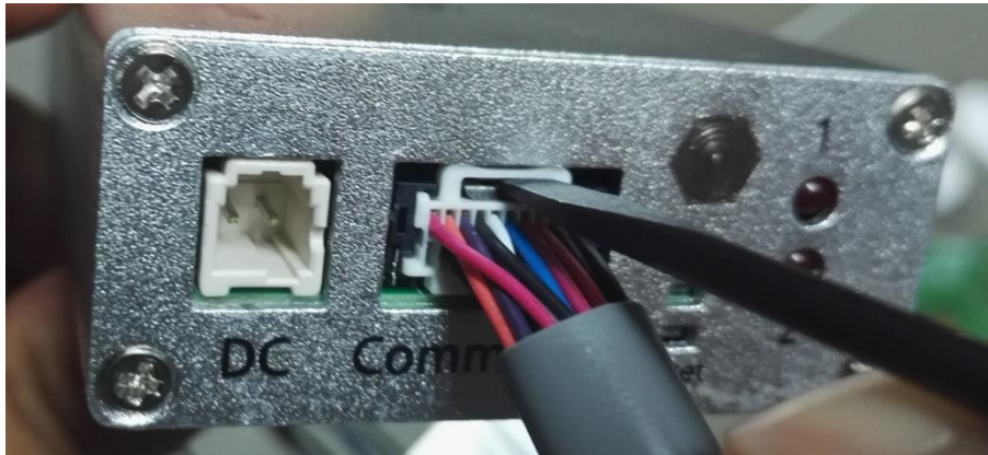
Figure 26 Uninstall the Cable
