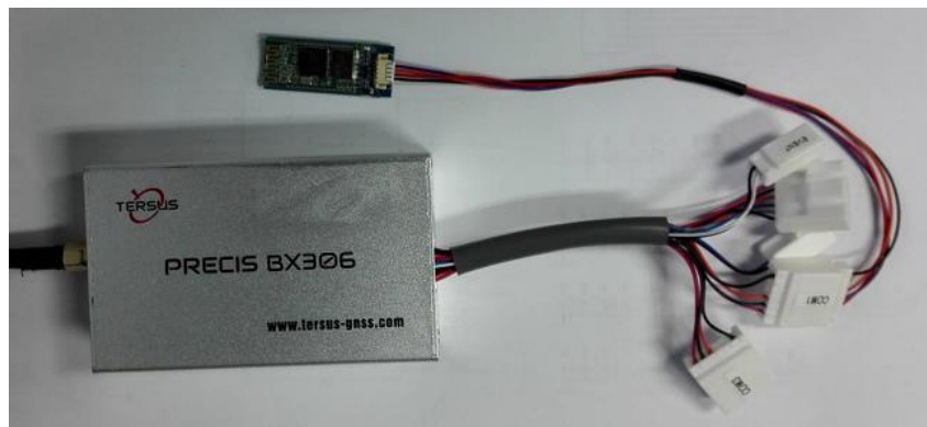
Figure 35 Outline of BX306 Connected to BT120
