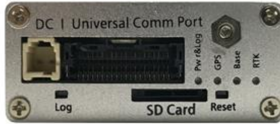
Figure 7 BX316 Enclosure Panel
