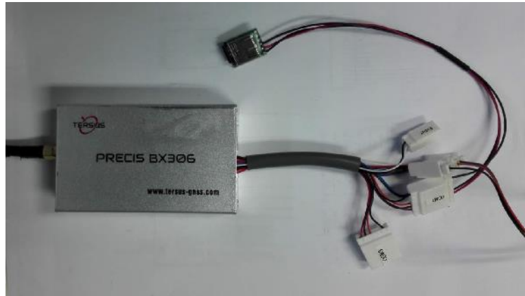
Figure 33 Outline of BX306 Connected to DL207
