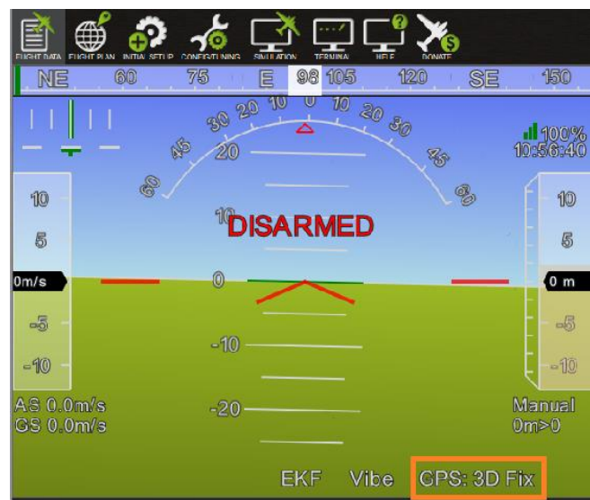
Figure 29 Pixhawk Get Position from BX306
