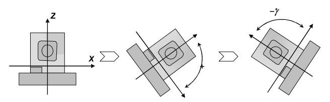
Fig.10.5. Rotation of a carrier with INS in roll
