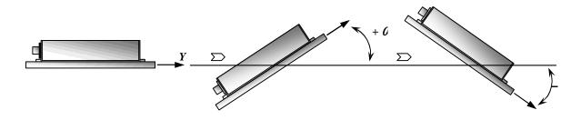
Fig.10.6. Rotation of a carrier with INS in pitch
