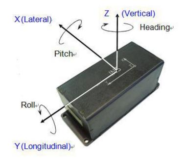
Fig.E.1. Coordinate system of the Tersus INS
