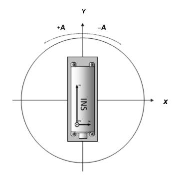
Fig.10.4. Rotation of a carrier object with INS in horizontal plane
