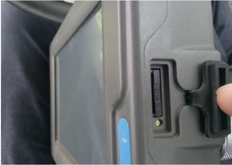
Figure 5 Remove the sealing rubber cover of SIM card slot
