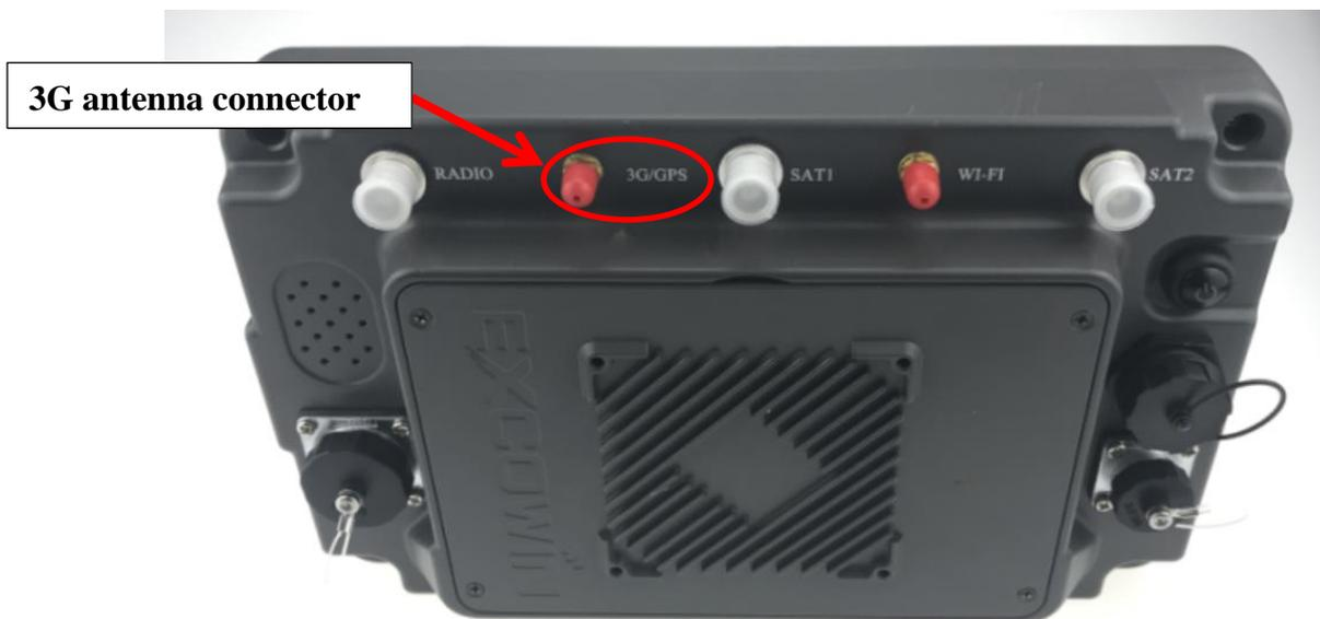
Figure 12 Back of tablet computer
