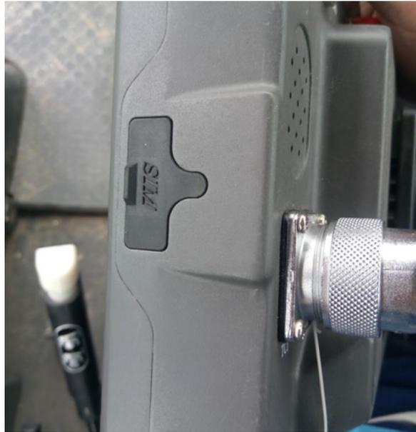
Figure 11 Fasten the sealing rubber cover of the slot
