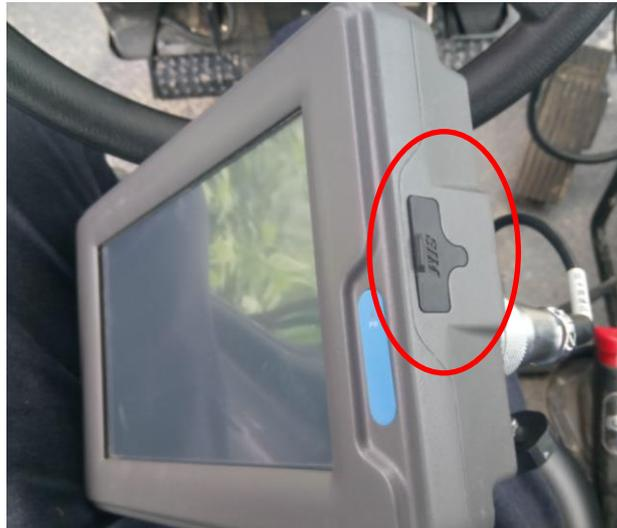
Figure 4 Sealing rubber cover of the SIM card slot
