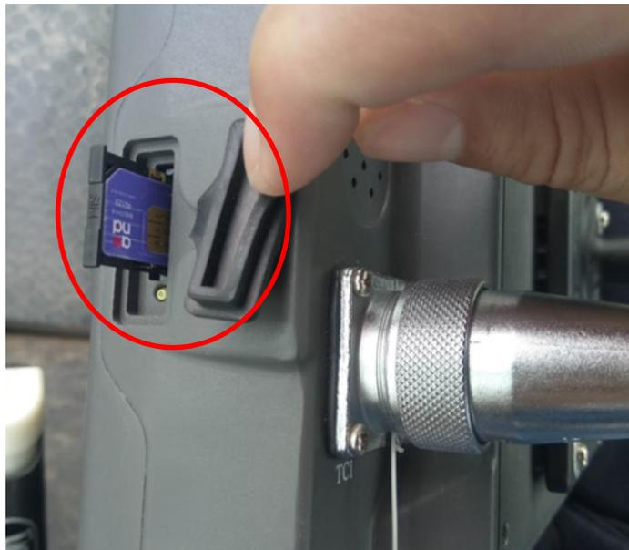
Figure 10 Insert the slot with SIM card into the tablet computer
