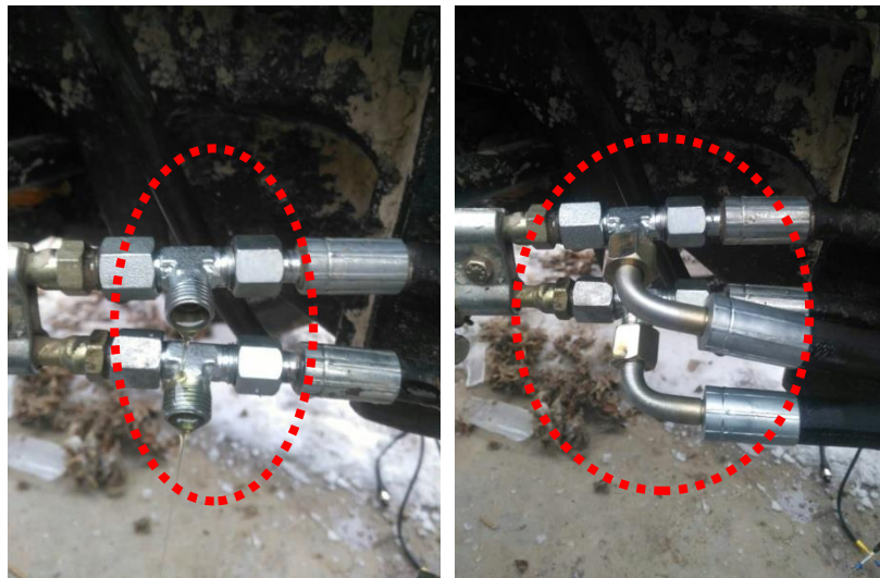
Figure 75 Disconnect existing connection at ports L/R/T of steering gear, connect a tee union, and then connect it to ports L/R/T of hydraulic valve
