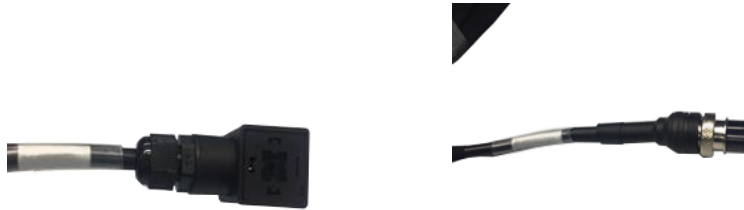
Figure 96 Battery connector (left) and power supply switch (right) of drive harness
