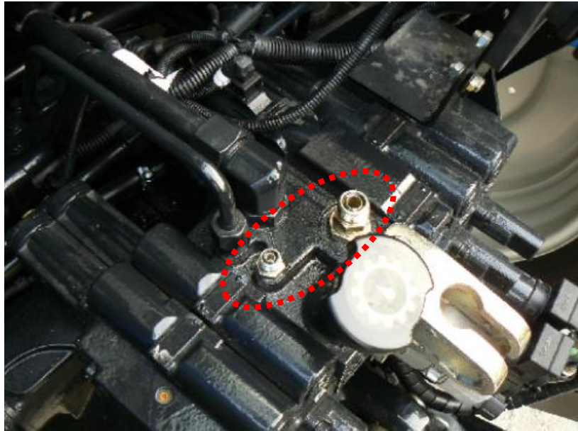
Figure 82 Replace the end caps of ports P and LS with transition union
