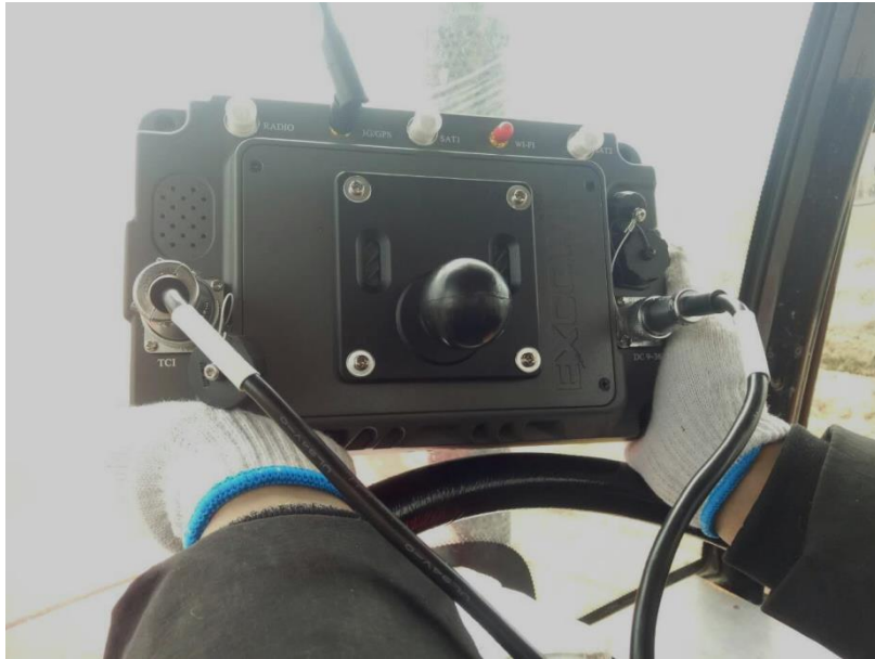
Figure 94 Connect data harness and panel computer
