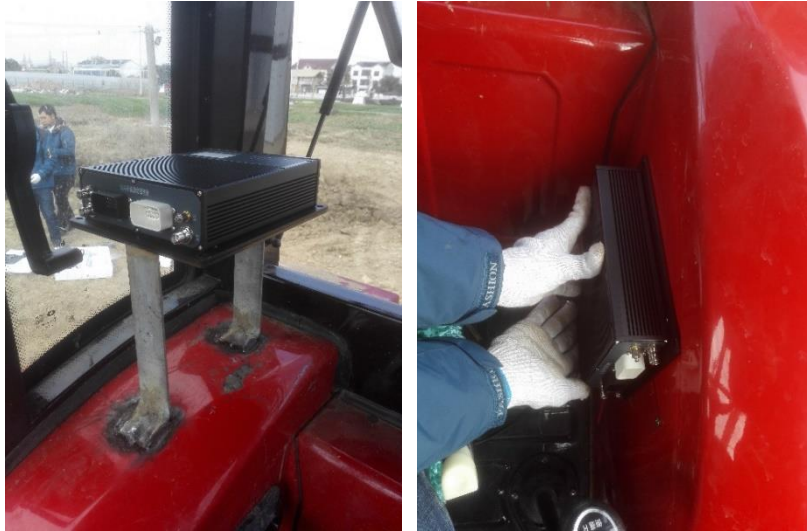
Figure 125 Main machine line outlet forward, LED light face upward (left); main machine line outlet forward, LED light face right (right)
