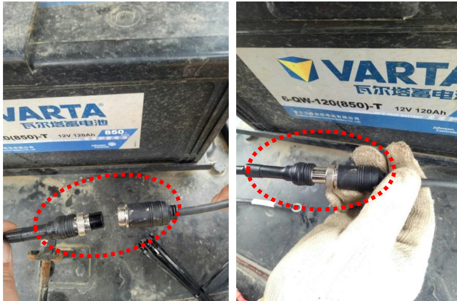
Figure 103 Connect pressure sensor terminal
