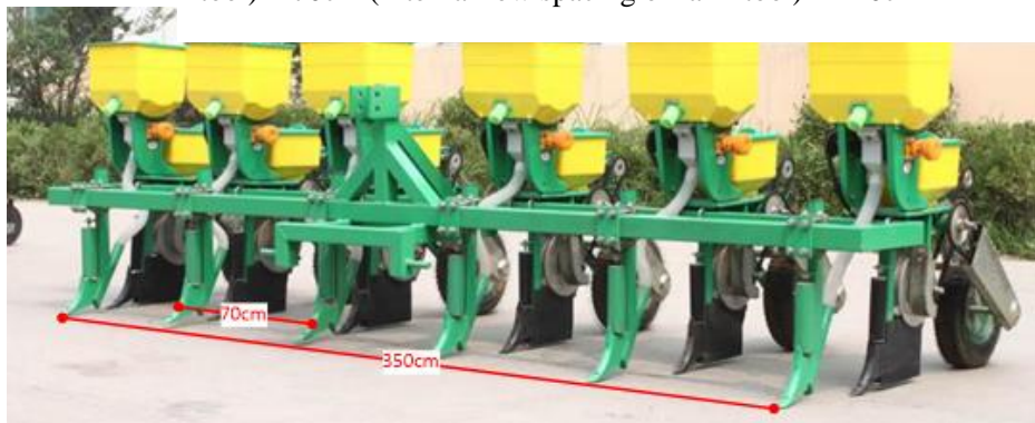
Figure 192 Operation width calculation of corn planter
