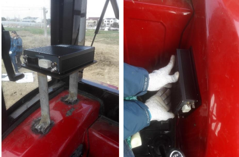
Figure 126 Main machine line outlet upward, LED light face forward (left); main machine line outlet upward, LED light face right (right)
