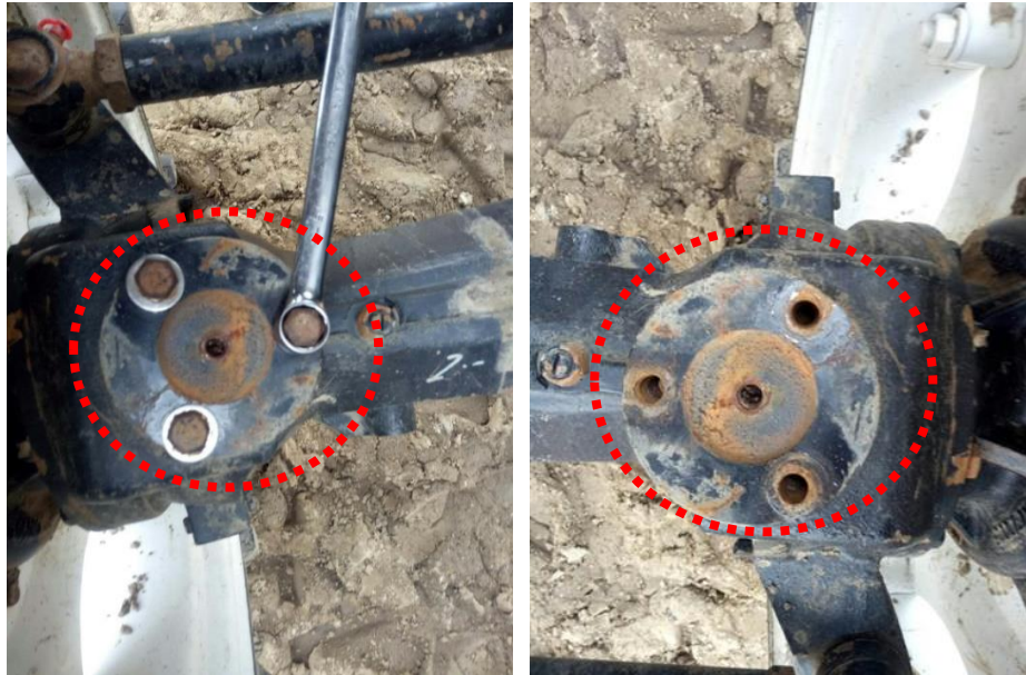
Figure 52 Remove the screws on the knuckle flange with a socket spanner
