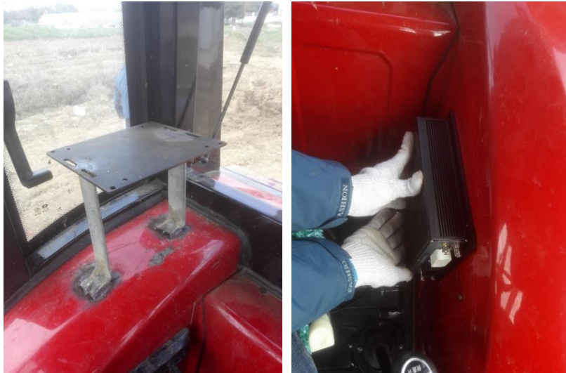
Figure 46 Proper installation position in the driving cab
