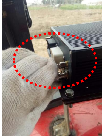
Figure 87 Connect radio antenna
