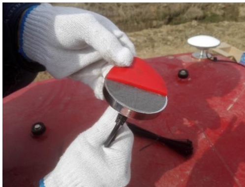
Figure 31 Press radio antenna to specified position with force
