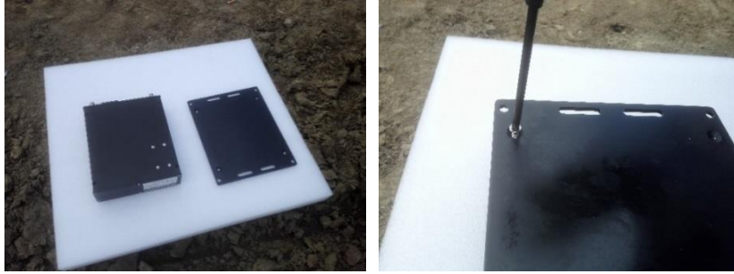
Figure 45 Connect the autopilot and the adapter plate with cross countersunk screws
