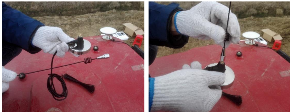
Figure 28 Assemble antenna mast and antenna pedestal
