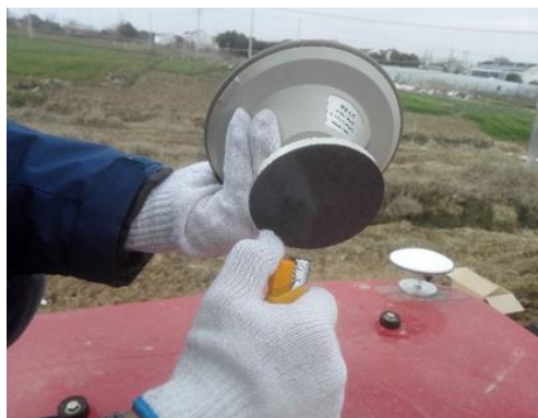
Figure 22 Heat the double faced adhesive tape in case of low temperature
