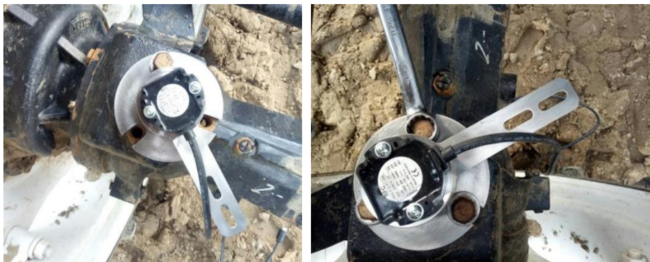
Figure 53 Place the assembled steering sensor onto the knuckle flange and secure it with original screws
