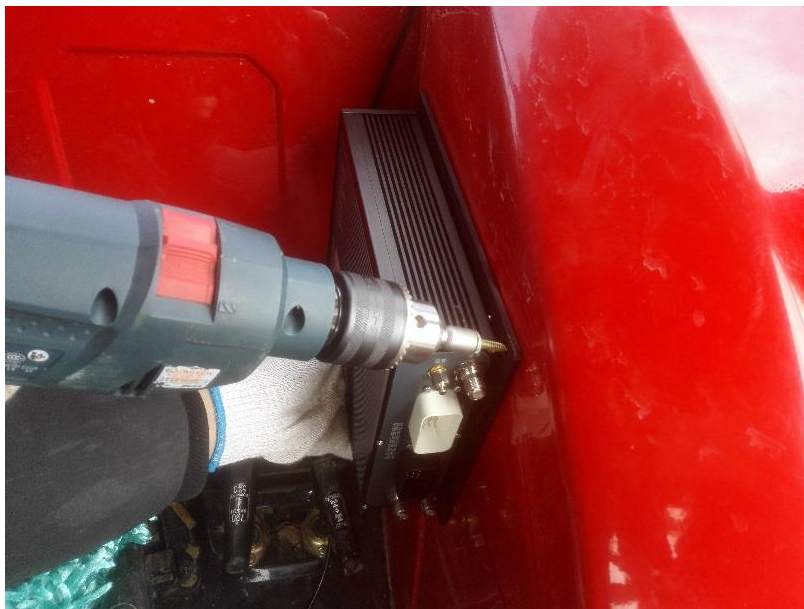
Figure 47 Fix the adapter plate to the installation surface with self-tapping screws and electric tool
