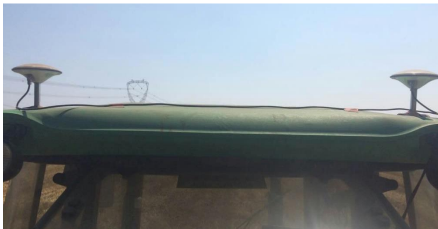
Figure 27 Route and bind the 3m RF cable at the driving cab top
