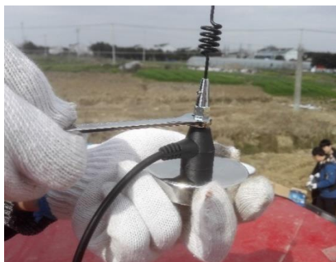
Figure 29 Tighten the antenna mast the antenna pedestal with wrench
