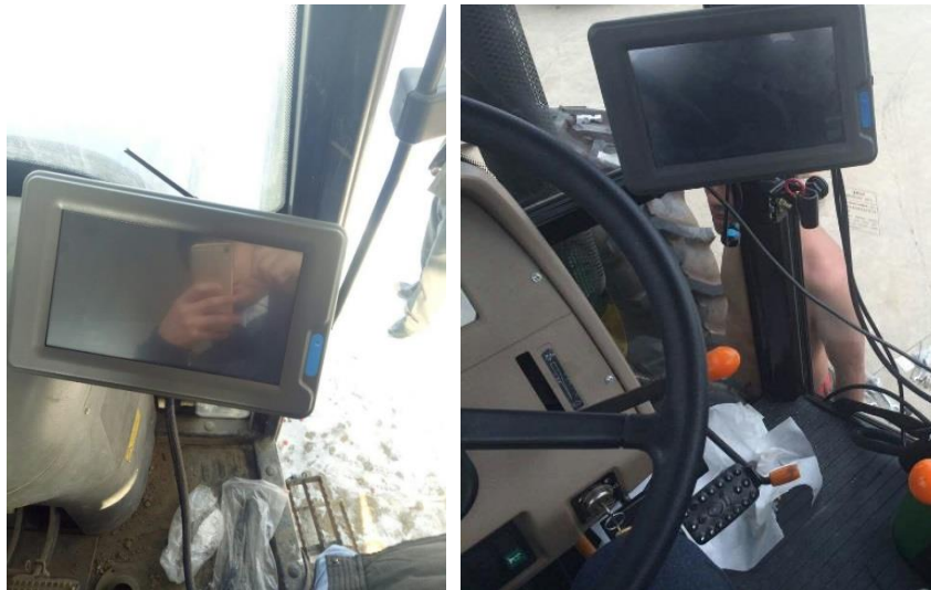
Figure 42 Panel computer properly installed
