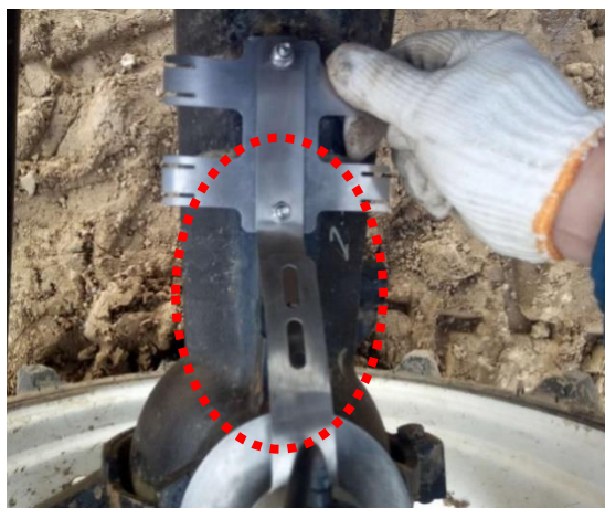
Figure 56 Connect the sensor stop plate and double cross stop frame and fix them with screws
