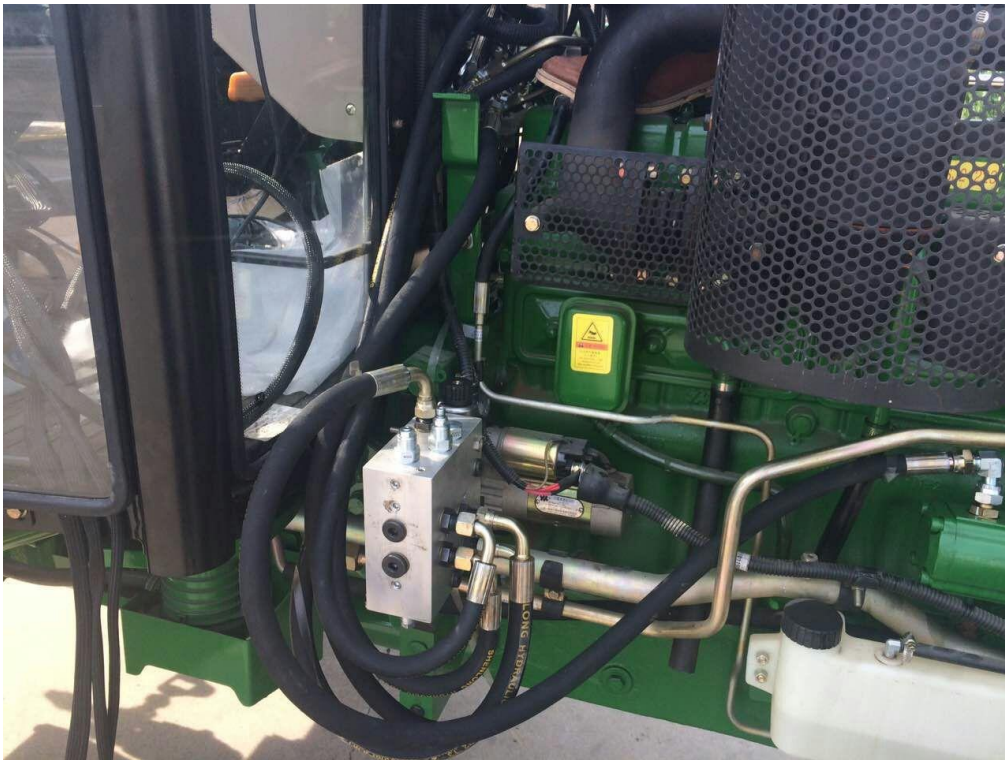
Figure 76 Sort out oil pipe
