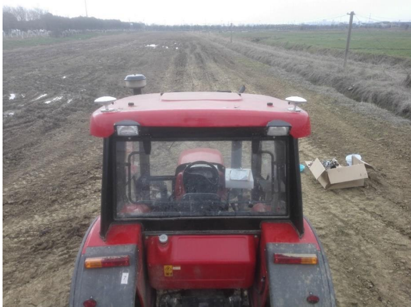
Figure 130 Example of lateral installation of antenna on the agriculture machine
