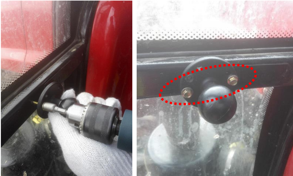
Figure 36 Fix the round plate knob of the panel computer bracket with electric tool and outer hexagon self-tapping screws
