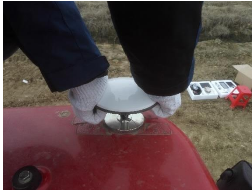
Figure 23 Press the antenna to specified position with force
