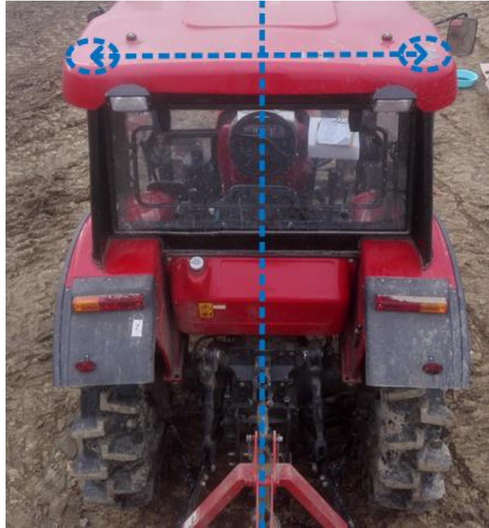
Figure 19 Ideal position of satellite navigation antenna on the vehicle (rear view)
