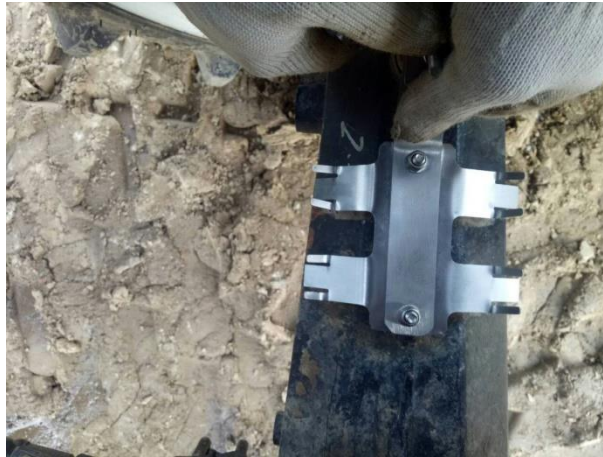
Figure 57 Remove the protective film of the double faced adhesive tape and press the double cross stop frame against the front axle
