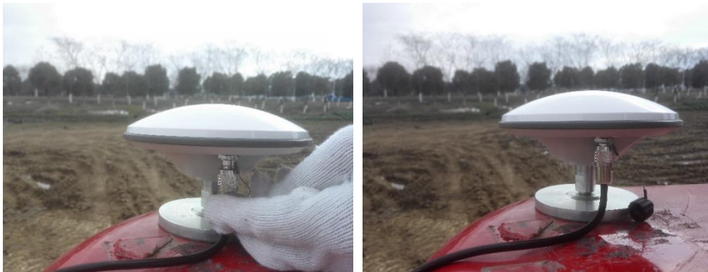
Figure 26 Tighten the 3M RF cable to the antenna (Do not use pliers or other tools to avoid damage to the connector)
