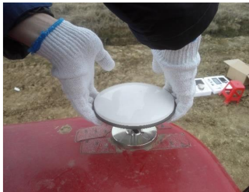
Figure 24 Slightly pull the antenna to check if it is securely fixed
