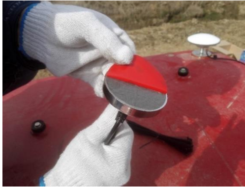
Figure 30 Remove the protective film of the double faced adhesive tape on the antenna pedestal
