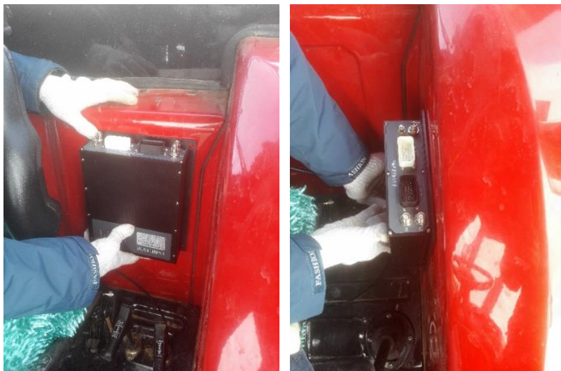
Figure 125 Main machine line outlet forward, LED light face upward (left); main machine line outlet forward, LED light face right (right)
