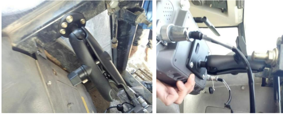
Figure 41 Connect the round plate knob and the rectangle knob with the link rod
