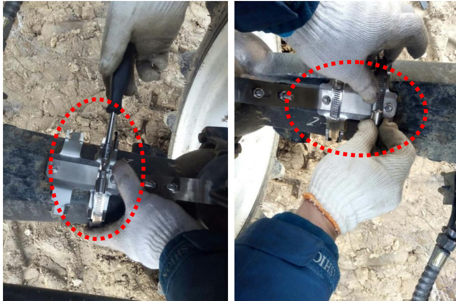
Figure 59 Bind and lock the double cross stop plate with anchor ear
