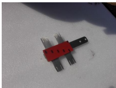
Figure 55 Adhere double faced adhesive tape to the lower part of the double cross stop frame (left) and bend the stop frame upward (right)
