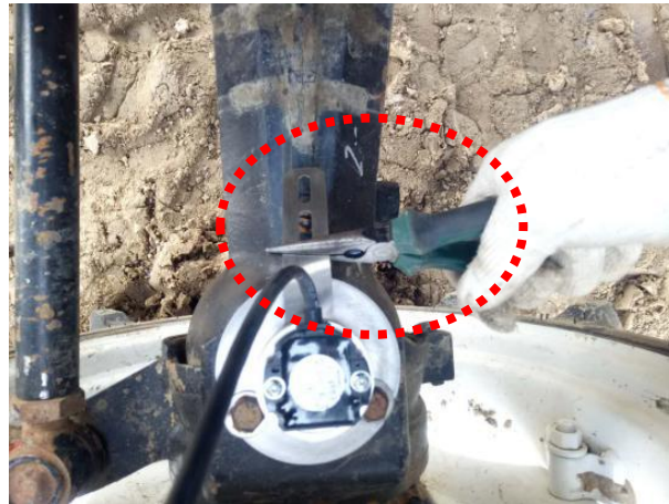
Figure 54 Bend the sensor stop plate downward
