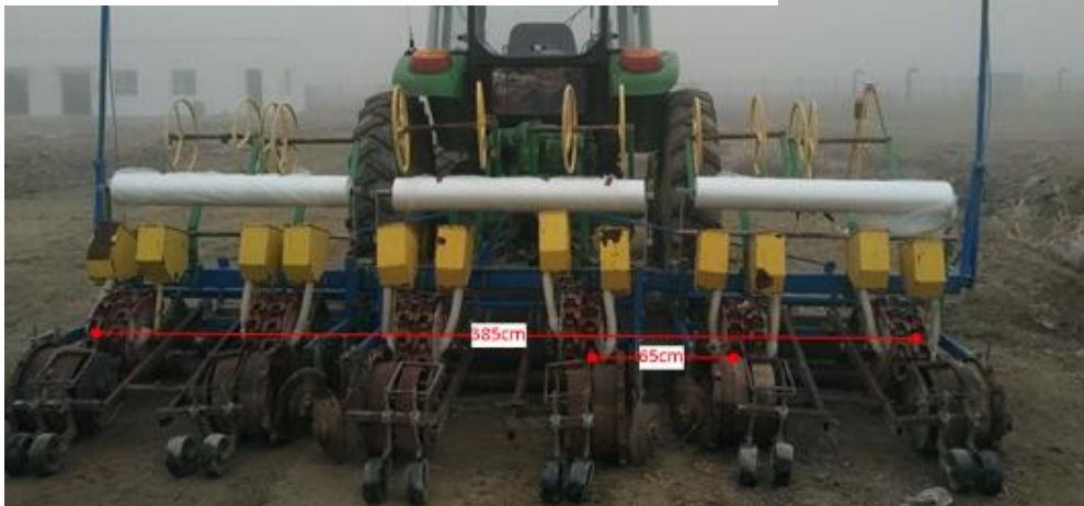
Figure 193 Operation width calculation of cotton planter
