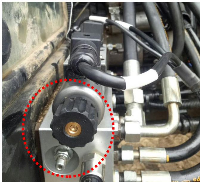
Figure 77 Start the engine and press the pressing points at both ends of the proportional valve to observe the actuation capability of the guide wheel
