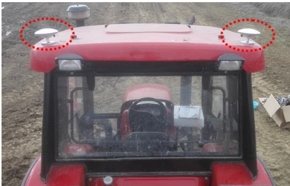
Figure 20 The satellite navigation antenna should be horizontally installed onto the vehicle with the RF connector at the inner side
