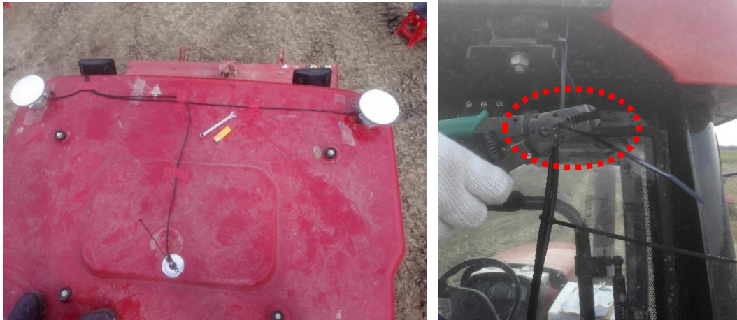
Figure 33 Fix and bind the RF cables on the driving cab top and lead them into the driving cab from the rear side window
