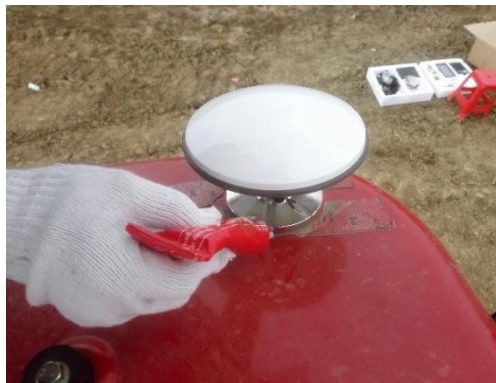
Figure 25 Apply waterproof sealant to the gap between antenna pedestal and vehicle top
