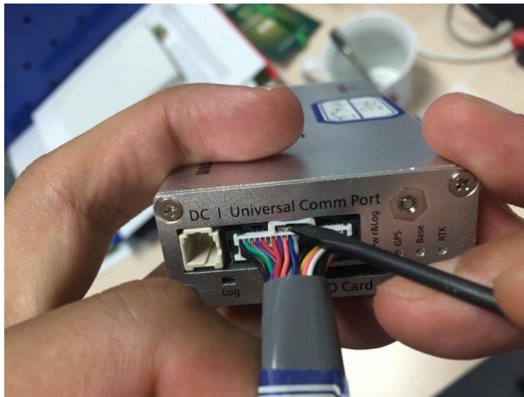
Figure 13 Uninstallation of the cable
