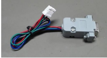
Figure 10 Serial level transfer cable
