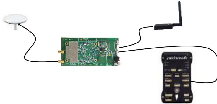
*Figure 29 Demonstration of Integration with Pixhawk autopilot*
