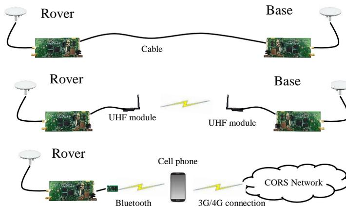
Figure 21 Three ways to connect to the base station data stream: wired connection (upper), UHF connection (middle)
