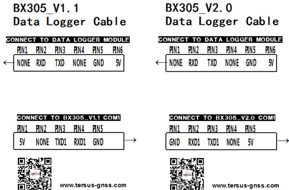
Figure 10 Labels of PreciS-BX305 V1.1 & V2.0 Data logger Cables
