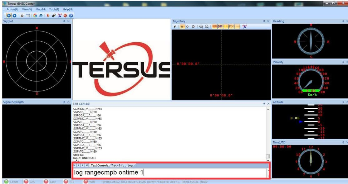
Figure 33 Enter commands for logging raw observation and broadcasting ephemeris data
