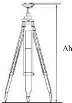
*Figure 31 Demonstration of antenna height measurement*
