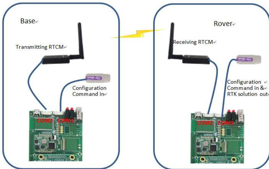
Figure 22 Overview of Tersus GNSS RTK Systems
