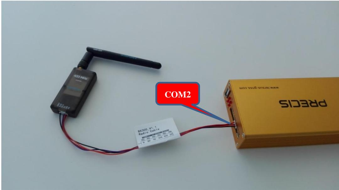
Figure 15 Connection between Pixhawk and Precis-BX305
