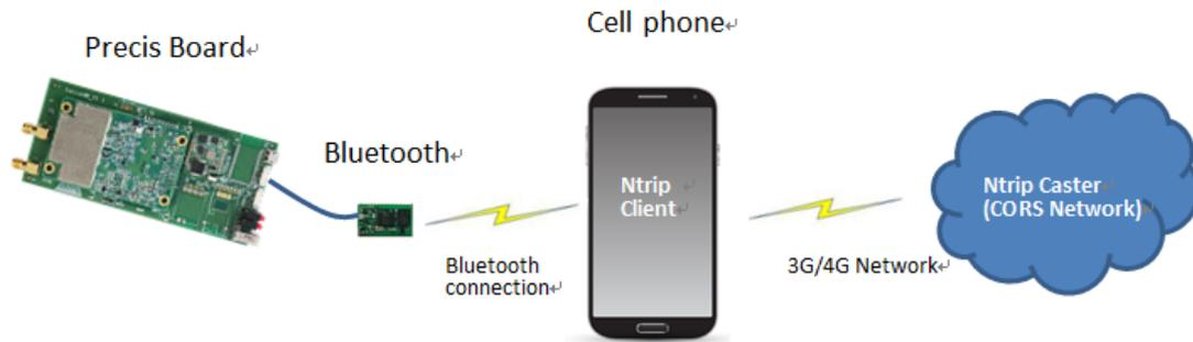
Figure 25 Demonstration of connecting Precis BX305 to CORS Network
