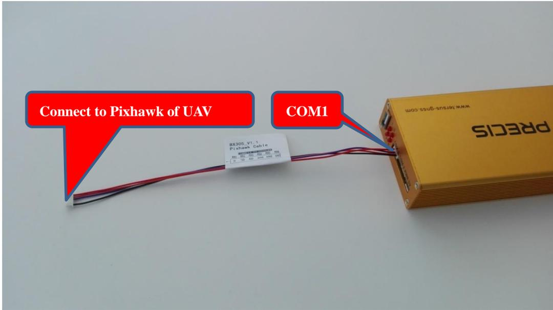
Figure 13 Connection between Pixhawk and Precis-BX305
