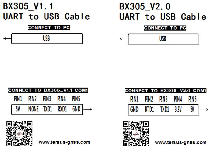
Figure 8 Labels of Preci-BX305 V1.1 & V2.0 UART\_To\_USB Converter Cables
