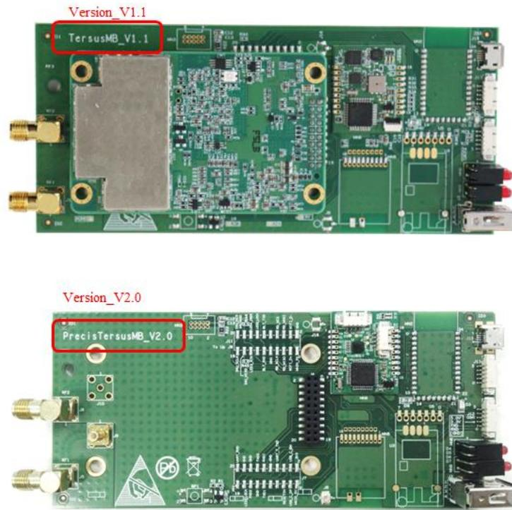
Figure 5 Identify Precis-BX305 V1.1 & V2.0 by Printed Labels
