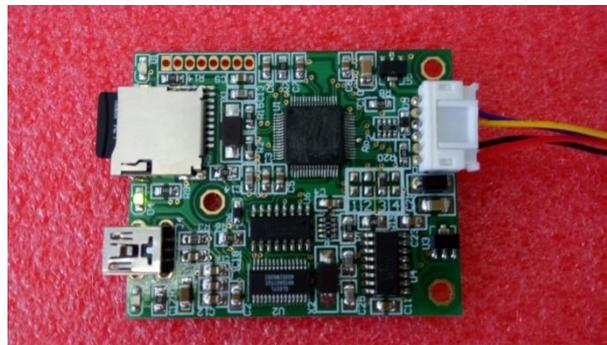
*Figure 32 External data logger*
