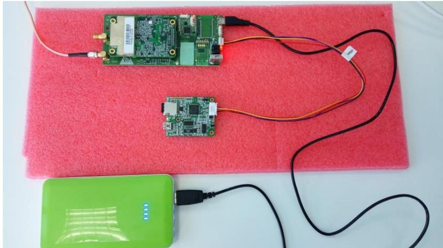
Figure 34 Connection of Precis-BX305, external data logger and power supplier
