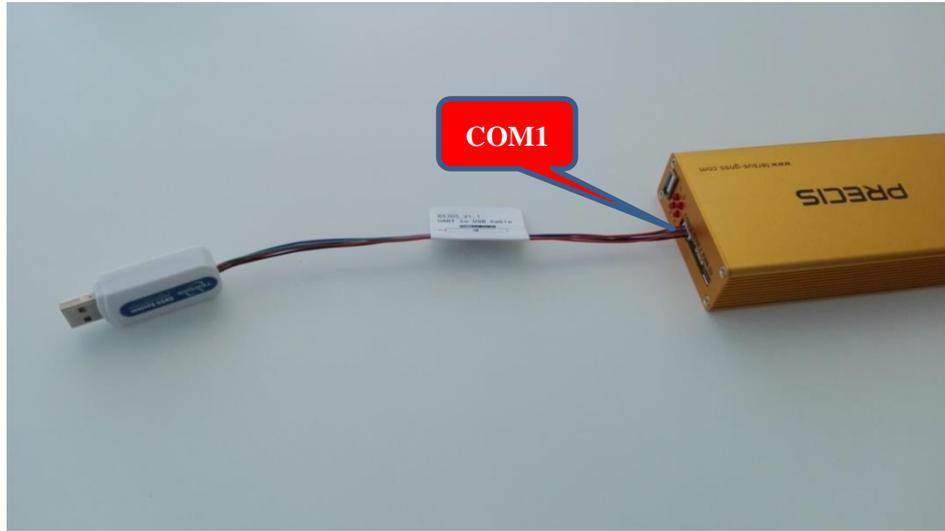
Figure 9 Connection between PreciS-BX305 and UART\_to\_USB Converter
