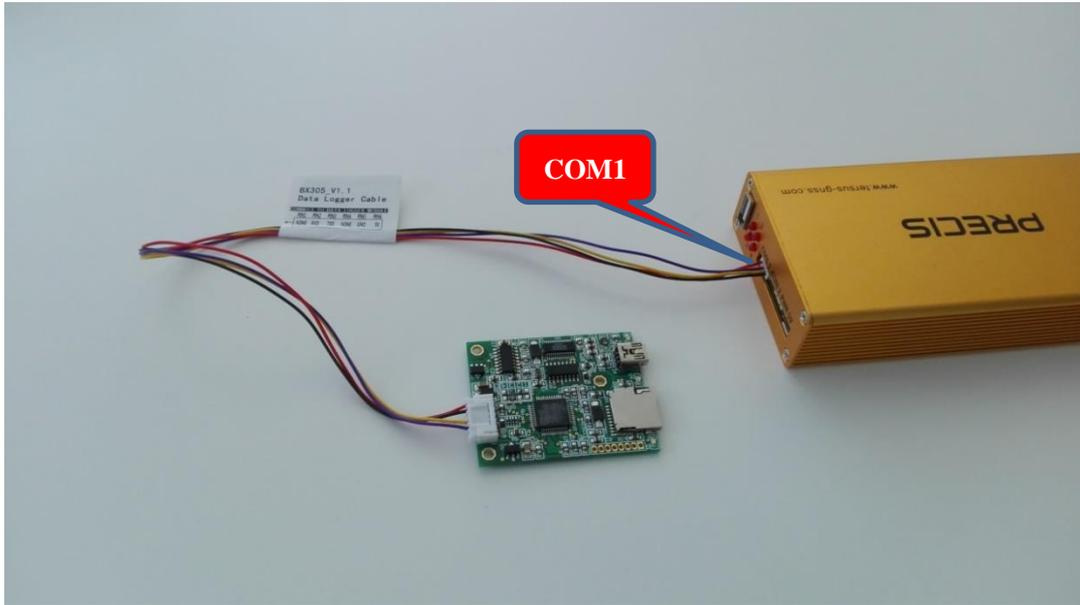
Figure 11 Connection between PreciS-BX305 and UART\_to\_Data Logger
