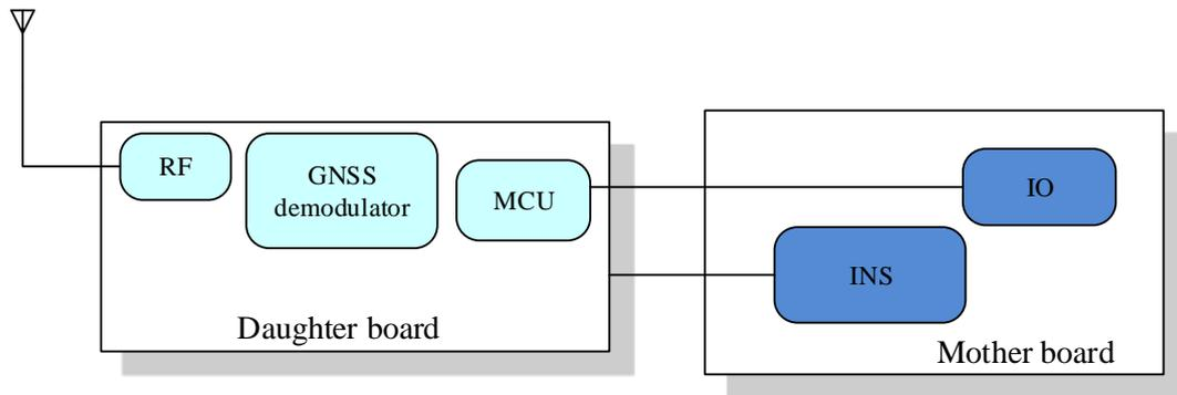
*Figure 2 System block diagram*
