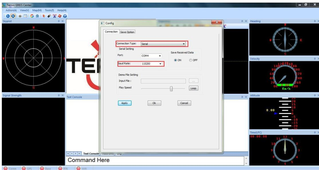
Figure 23 Establish Serial Connection with Tersus GNSS Center
