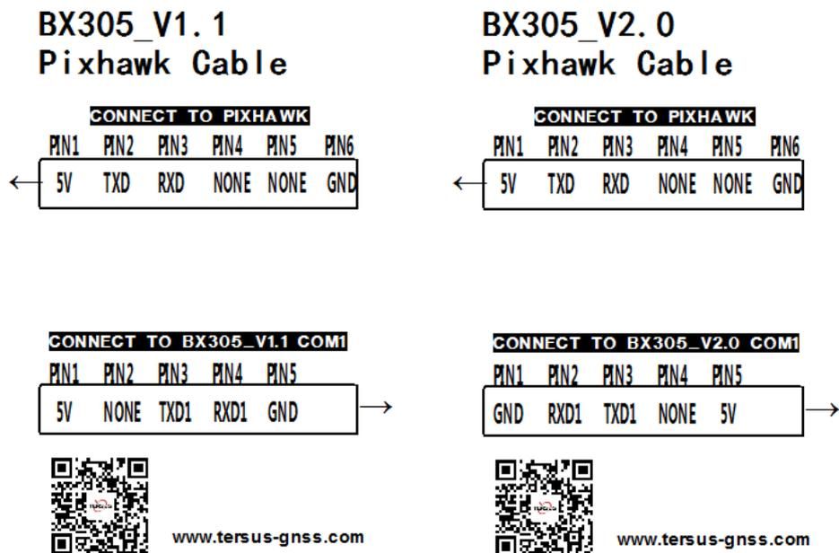
Figure 12 Labels of PreciS-BX305 V1.1 & V2.0 Pixhawk Cables
