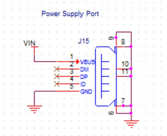
Figure 6 Schematic of Internal Micro\_USB Connector
