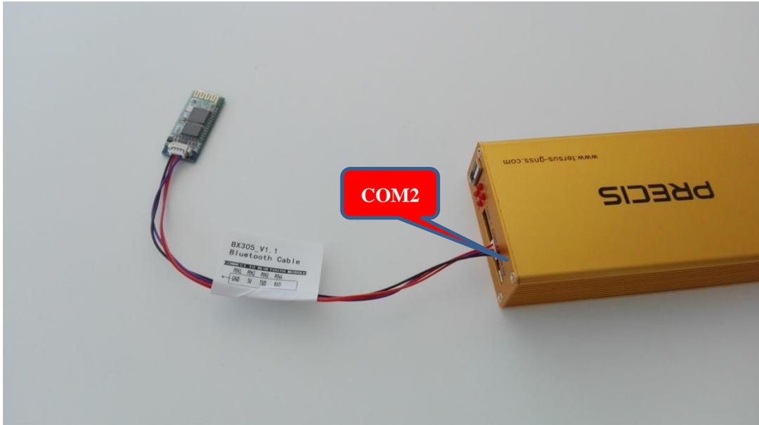
Figure 17 Connection between Bluetooth module and Precis-BX305
