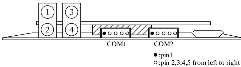
Figure 7 Back Panel View of Precis-BX305 Board
