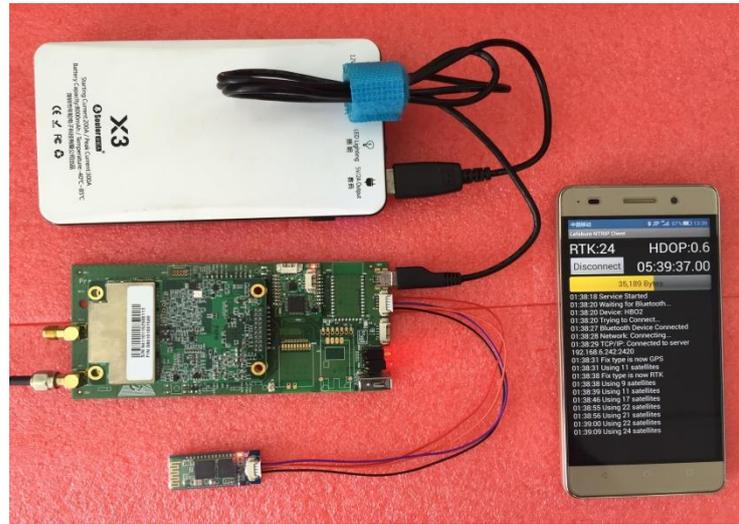
Figure 26 Demonstration of connecting Bluetooth module, mobile phone, PreciS-BX305 and supply supplier
