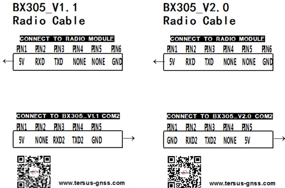
Figure 14 Labels of Precis-BX305 V1.1 & V2.0 Radio Cables
